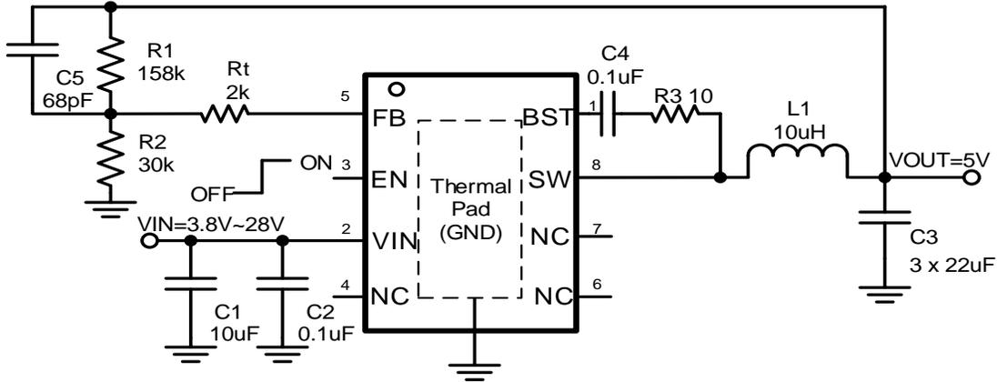
\*For input voltage higher than 18V, R3=10 is highly recommend.
