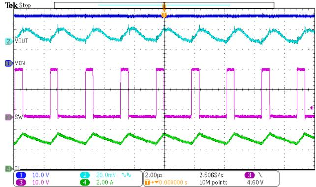
Figure 13. SW node waveform and Output Ripple
