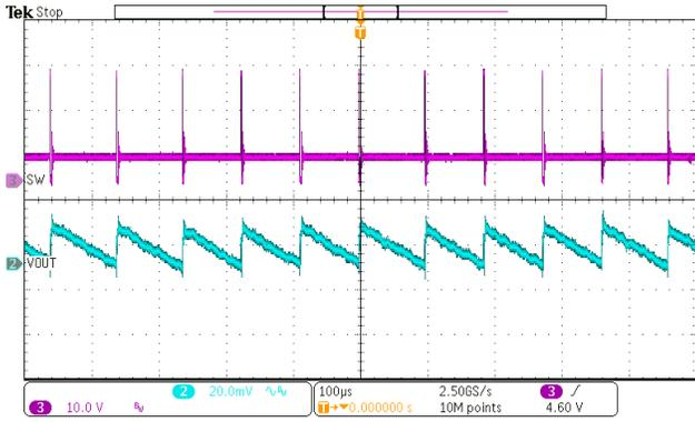
Figure 12. SW node waveform and Output Ripple
