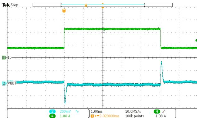
Figure 16. Load Transient
