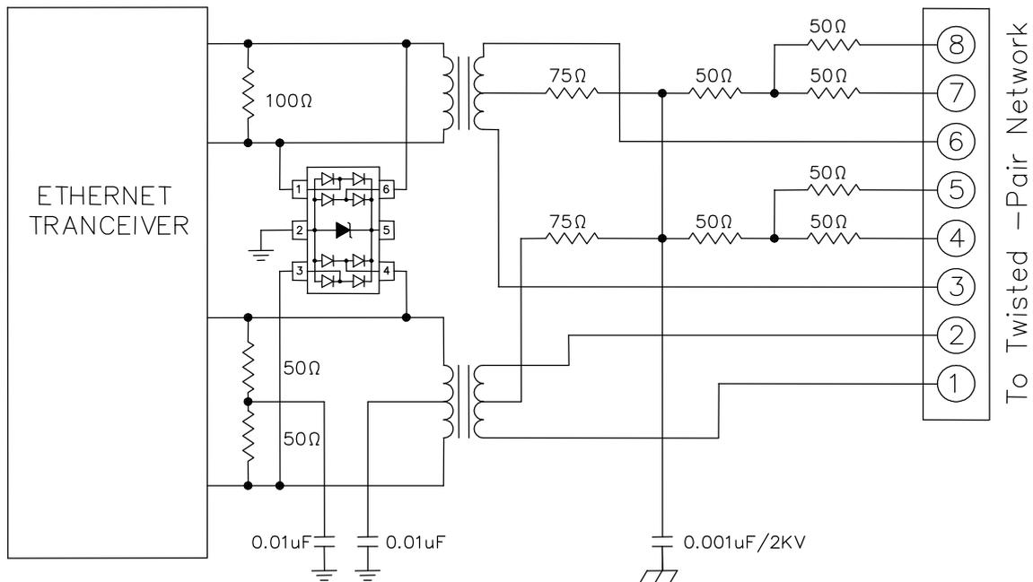
Figure 9 - 10/100 Ethernet Differential and Common Mode Protection
