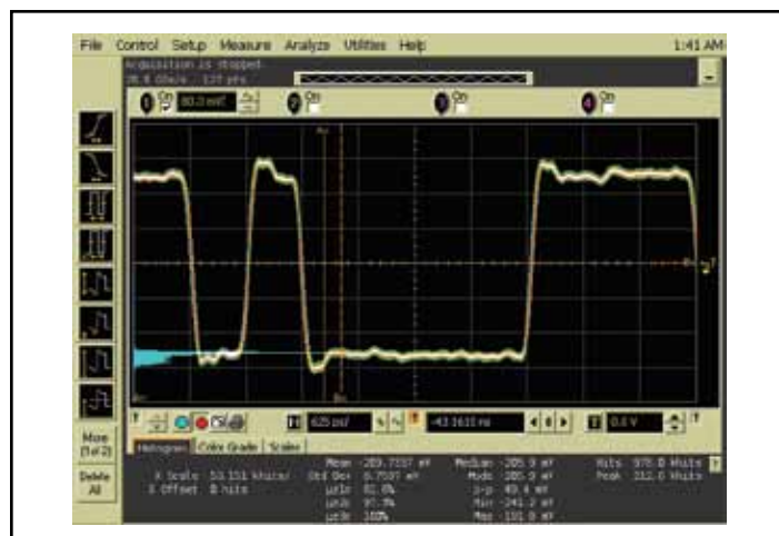
Output Waveform (400mV, 0dB pre-emphasis)
