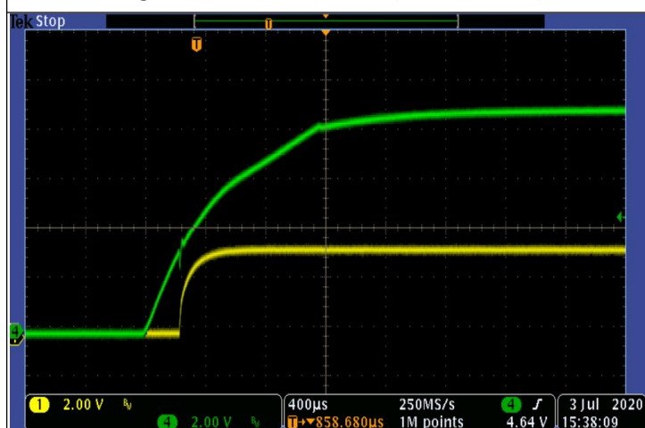
Fig 7 Vout Load Transient (50 to 250mA)
