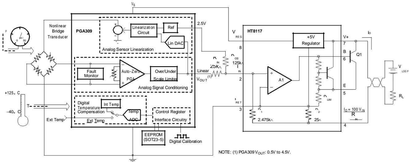
**Figure 5. Complete 4-20mA Pressure Transducer Solution with PGA309 and HT8117C**
