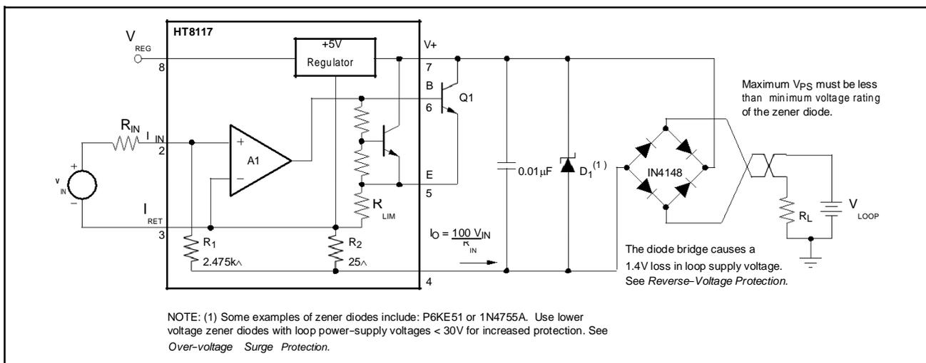
**Figure 3. Reverse Voltage Operation and Over-Voltage Surge Protection**
