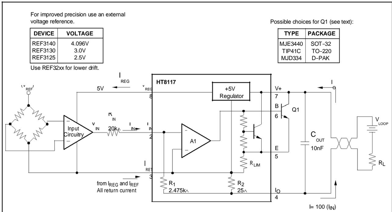
**Figure 1. Basic Circuit Connections**
