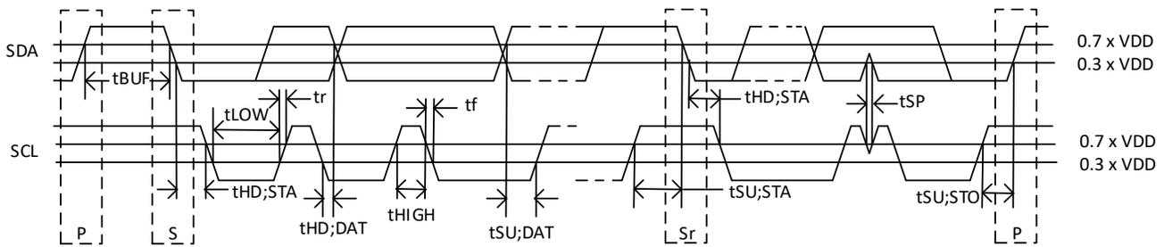
Fig 3. Definition of timing on I<sup>2</sup>C-bus
