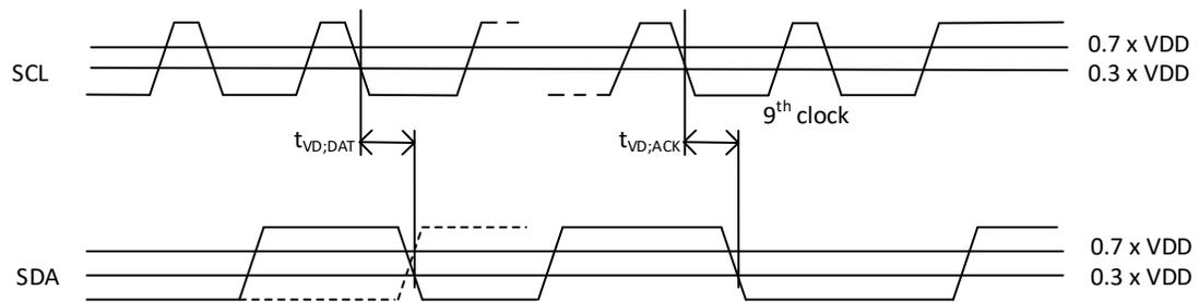
Fig 20. Parameter Measurement Waveform:  $t_{VD;DAT}$  &  $t_{VD;ACK}$
