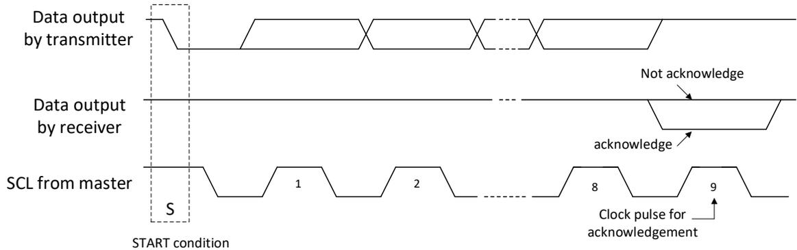
Fig 15. Acknowledgement on I<sup>2</sup>C-bus
