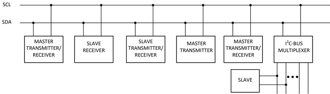
Fig 14. System configuration
