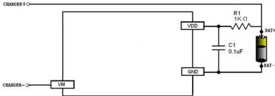
**Fig 6 XB7608AJL in a Typical Battery Protection Circuit**
