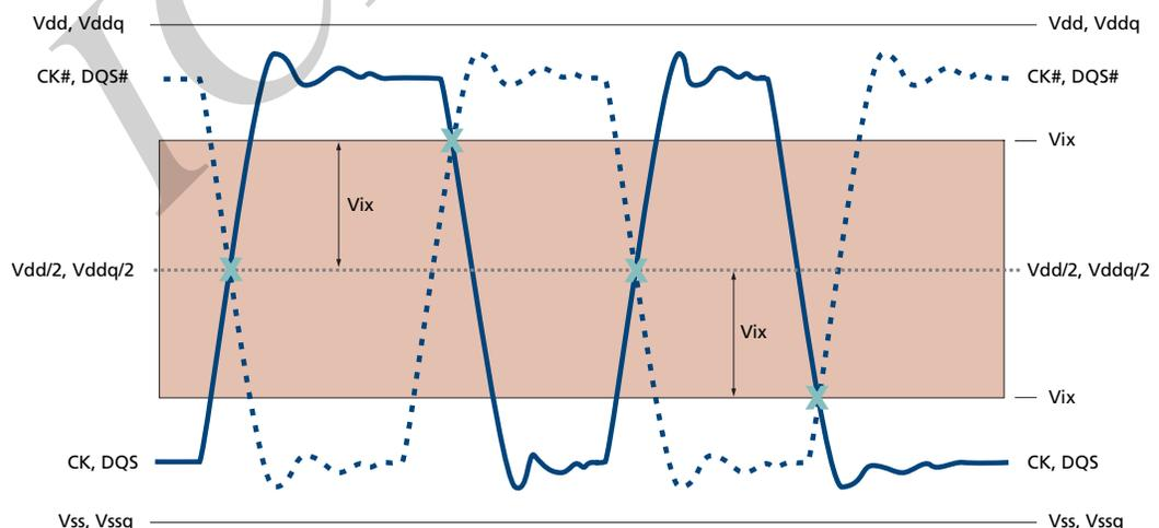
**Figure 18: Single-Ended Requirements for Differential Signals**
