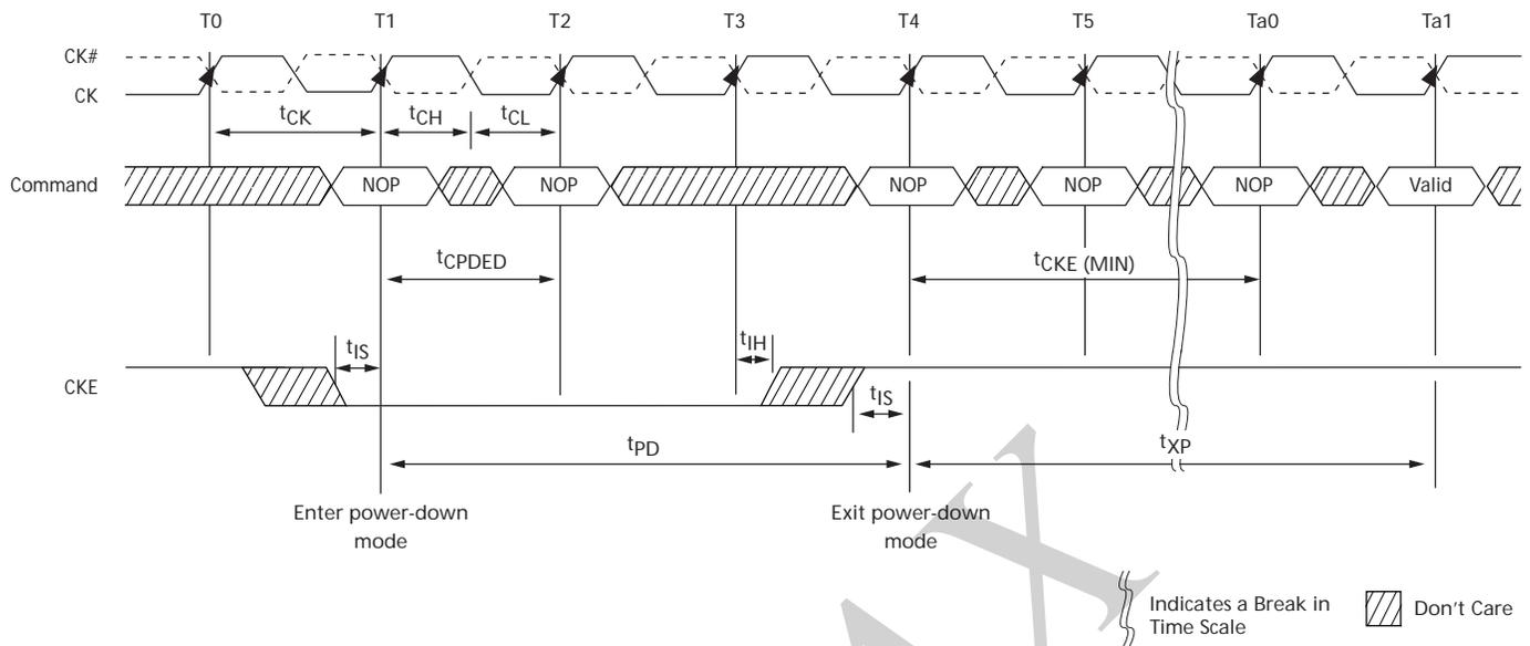
Figure 98: Precharge Power-Down (Slow-Exit Mode) Entry and Exit
