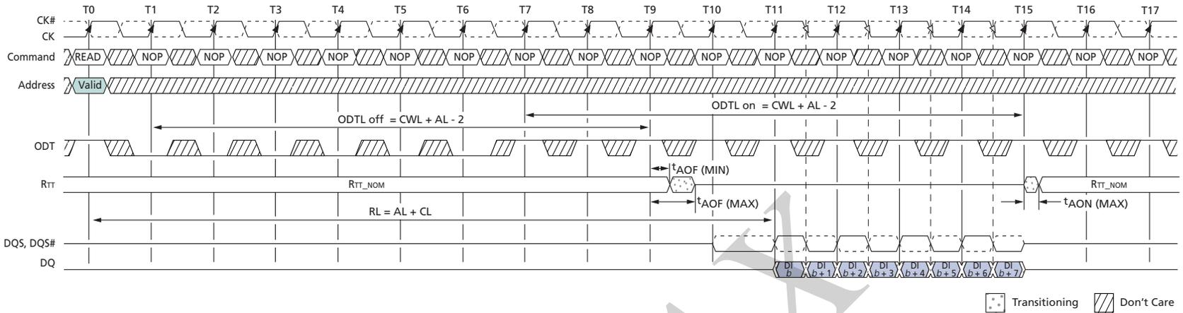
Notes: 1. ODT must be disabled externally during READs by driving ODT LOW. For example, CL = 6; AL = CL - 1 = 5; RL = AL + CL = 11; CWL = 5; ODTL on = CWL + AL - 2 = 8; ODTL off = CWL + AL - 2 = 8. Rtt\_NOM is enabled. Rtt\_WR is a "Don't Care."
