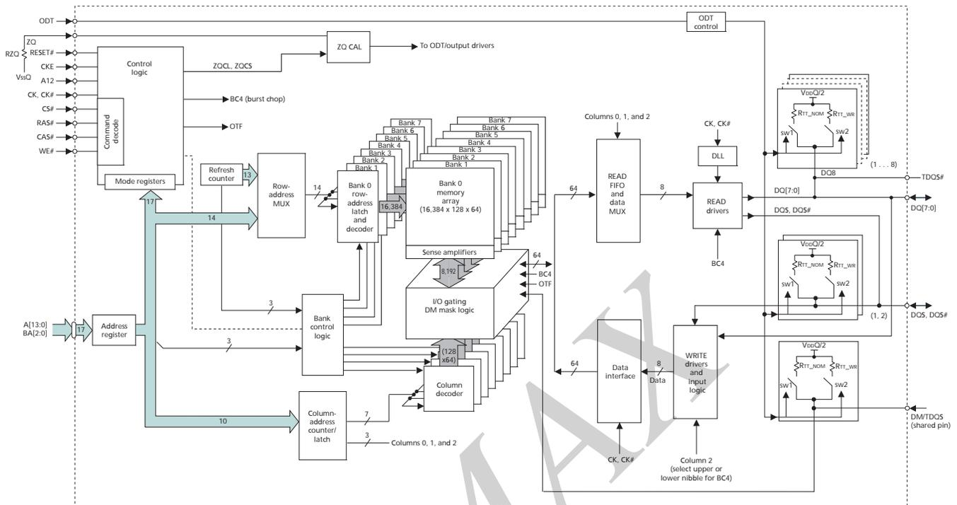
Figure 4: 64 Meg x 16 Functional Block Diagram
