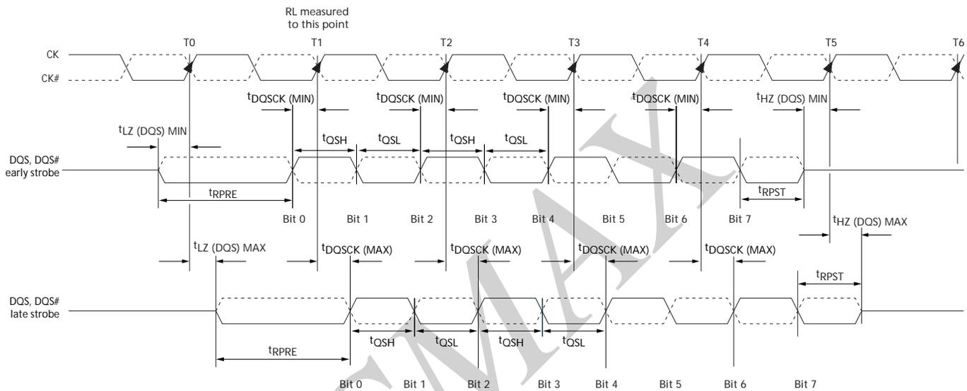
Figure 79: Method for Calculating  $t_{LZ}$  and  $t_{HZ}$
