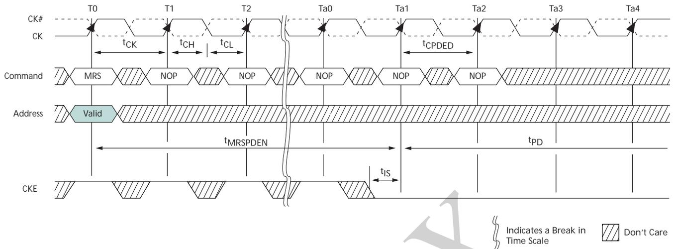
Figure 106: Power-Down Exit to Refresh to Power-Down Entry
