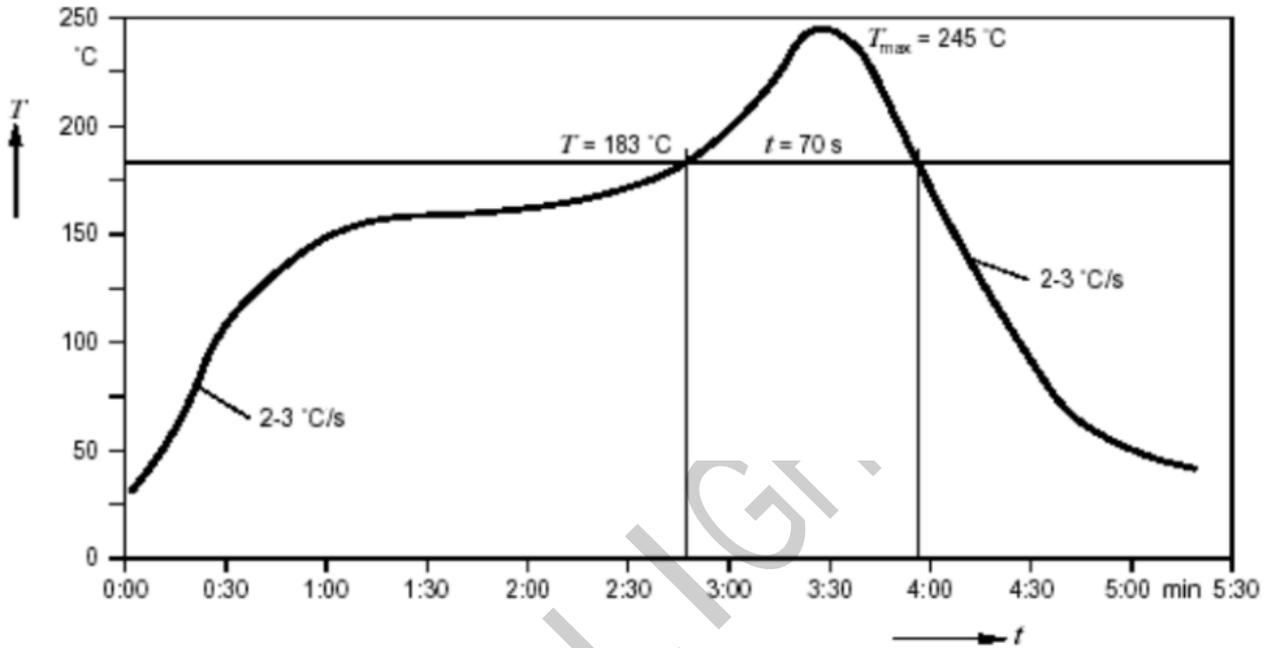
● Suggest Pb-Free IR Reflow Soldering Profile Condition:
