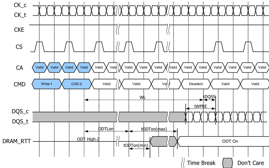
**Figure - Asynchronous ODT<sub>OFF</sub> Timing Example, tWPRE = 2 nCK, tDQSS = Nominal**
