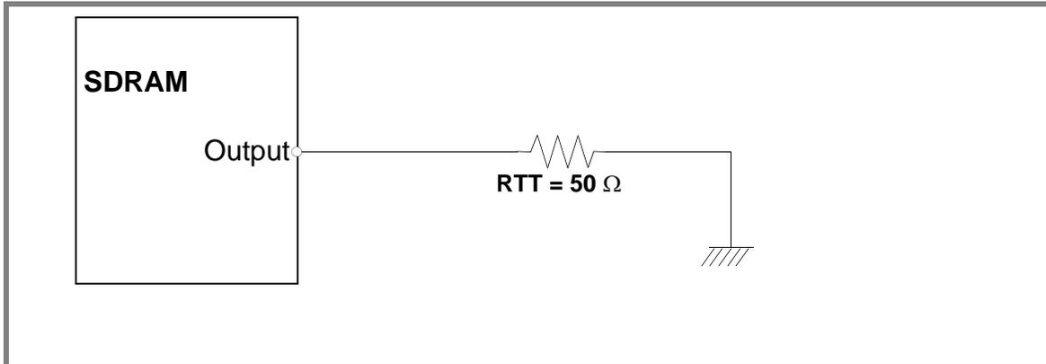
Note: 1. All output timing parameter values (like  $t_{DQSQ}$ ,  $t_{DQSQ}$ ,  $t_{QHS}$ ,  $t_{HZ}$ ,  $t_{RPRE}$  etc.) are reported with respect to this reference load. This reference load is also used to report slew rate.
