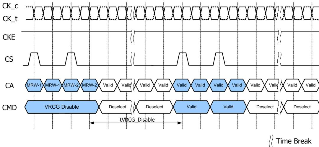
Note that LPDDR4 SDRAM devices support Vref(CA) and Vref(DQ) range and value changes without enabling VRCG high current mode.
