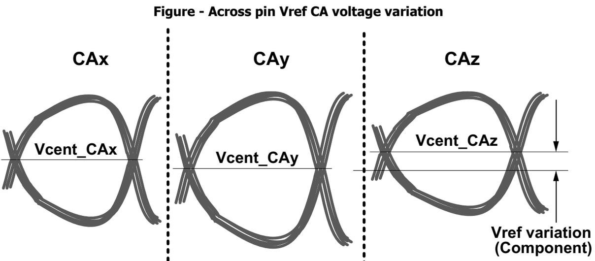
Vcent\_CA(pin avg) is defined as the midpoint between the largest Vcent\_CA voltage level and the smallest Vcent\_CA voltage level across all CA and CS pins for a given DRAM component. Each CA pin Vcent level is defined by the center, i.e. widest opening, of the cumulative data input eye as depicted in the above figure. This clarifies that any DRAM component level variation must be accounted for within the DRAM CA Rx mask. The component level Vref will be set by the
