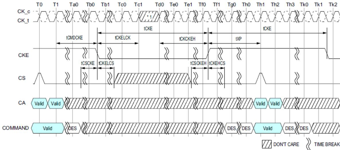
1. Input clock frequency can be changed or the input clock can be stopped or floated during power-down, provided that upon exiting power-down, the clock is stable and within specified limits for a minimum of  $RU(t_{CKCKEH}/t_{CK})$  of stable clock prior to power-down exit and the clock frequency is between the minimum and maximum specified frequency for the speed grade in use.
