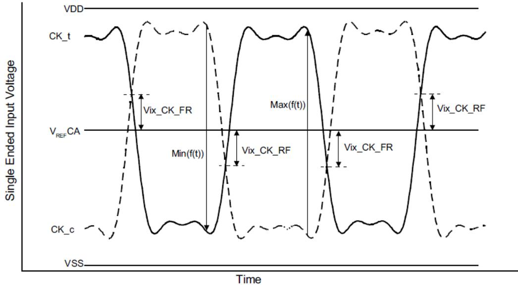
NOTES : 1. The base level of Vix\_CK\_FR/RF is  $V_{REF\_CA}$  that is LPDDR4 SDRAM internal setting value by  $V_{REF\_Training}$ .
