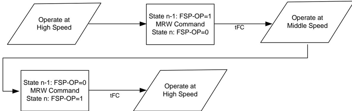
Switching to a third (or more) Set-Point can be accomplished if the memory controller has stored the previously-trained values (in particular the Vref-CA calibration value) and re-writes these to the alternate Set-Point before switching FSP-OP (Figure below).
