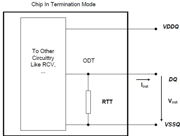
**Table - ODT DC Electrical Characteristics, assuming  $R_{ZQ} = 240\Omega \pm 1\%$  over the entire operating temperature range after a proper ZQ calibration for up to 3200Mbps.**
