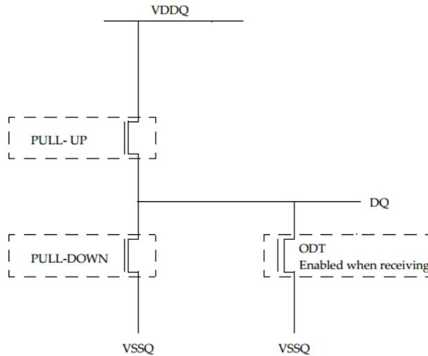
To ensure that the target impedance is achieved the LVSTL I/O cell is designed to be calibrated as following procedure.
