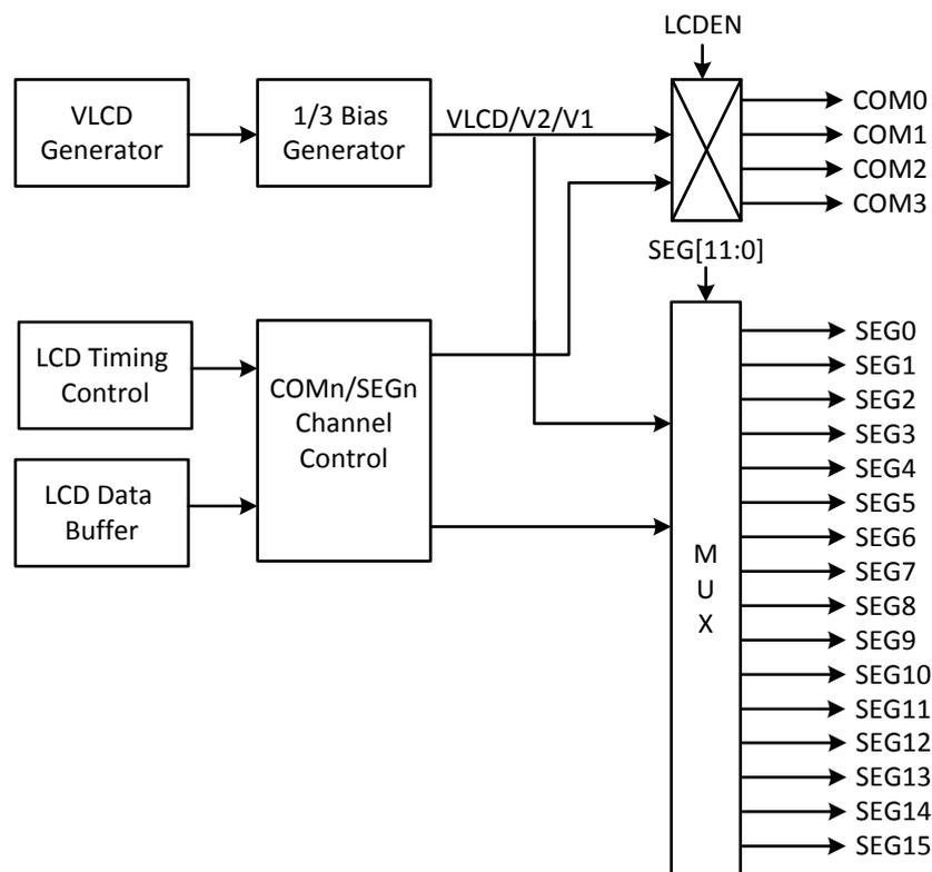
In LCD mode, the LCD builds in one internal bias circuit to adjust LCD power and bias voltage. There are 16-pin GPIO shared with COM pins and SEG pins which controlled by LCDSEG and LCDSEG1 registers. The LCD builds in P0CON/P1CON/P2CON/P3CON registers to set pure analog input pin. After setup LCDEN bit, the LCD starts output analog data. In static mode, the selected COM/SEG pins switch to like GPIO output mode and only output 0V and VDD voltage.
