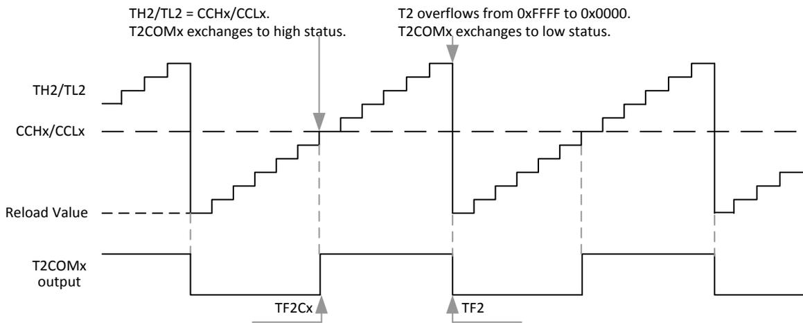
By contrast, the indirectly output method is an event which keep the mapped pin's previous output setting until Timer 2 counter overtakes CRC/CC1/CC2/CC3 register value. In this mode, the transition of the output signal can be configured by software. In other word, the P0.0 register bit would be affect T2COM0/P0.0 pin when TH2/TL2 equal to CRC registers. A Timer 2 overflow causes no output change.
