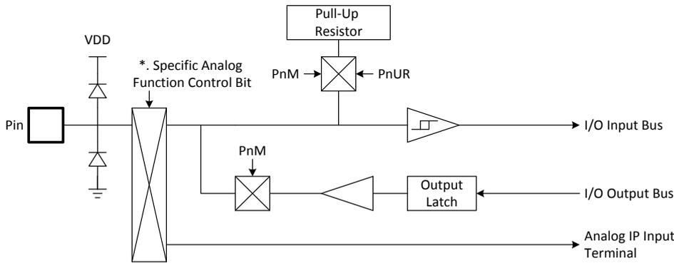
\*. Some specific functions switch I/O direction directly, not through PnM register.
