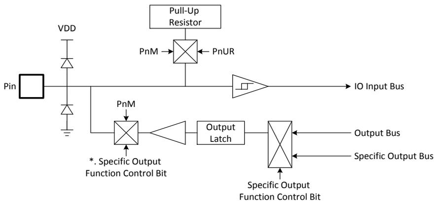
\*. Some specific functions switch I/O direction directly, not through PnM register.
