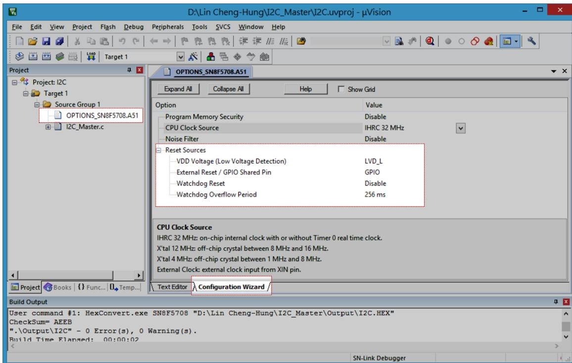
The code option is the system hardware configurations including oscillator type, noise filter option, watchdog timer operation, LVD option, reset pin option and flash ROM security control. The code option items are as following table:
