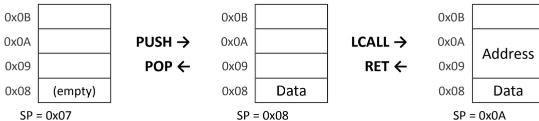
By default, stack pointer (SP register) points to 0x07 which means the stack area begin at IRAM address 0x08. In other word, if a planned stack area is assigned from IRAM address 0xC0, the appropriate SP register is anticipated to set at 0xBF after system reset.
