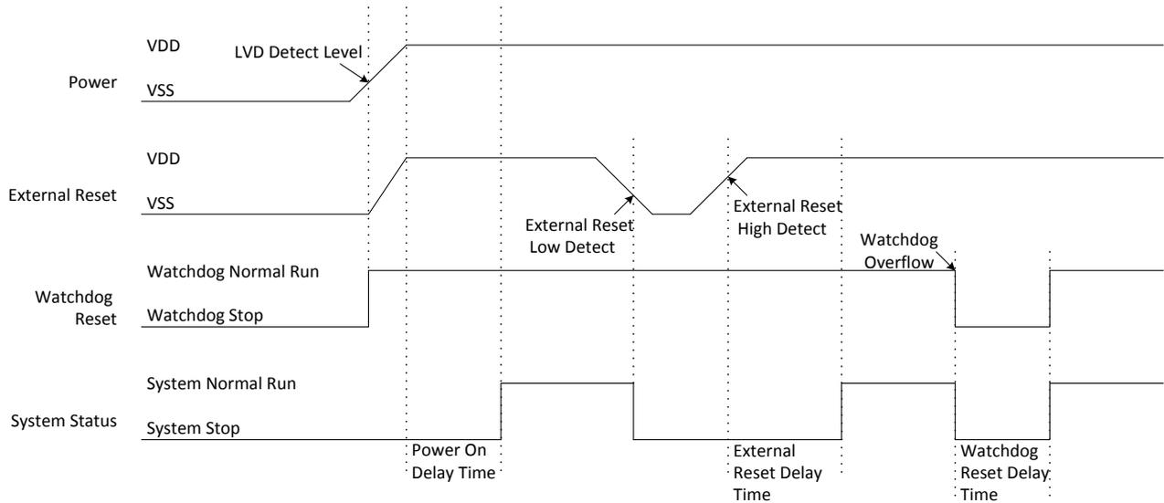
The power stabilization period spends 4.6 ms in typical condition. Afterward the microcontroller fetches CPU Clock Source selection automatically. The selected clock source would be driven, and the system counts 2048 times of the clock period and 5 times of the internal low-speed oscillator clocks to ensure its reliability.
