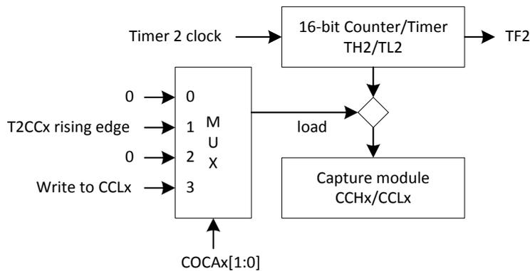
The split event can from hardware or software. The T2CC0 pin (shared with P0.5) can trigger a hardware split event that duplicates TH2/TL2 value to CRCH/CRCL registers, whereas T2CC1 (P0.6), T2CC2 (P0.2) and T2CC3 (P0.3) respectively control CC1 to CC3 registers.
