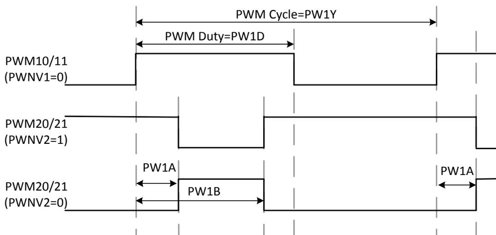
The PWM dead band occurs in PWM high pulse width, and the dead band period is programmable from PW1A and PW1D-PW1B registers. The dead band period is symmetrical at left-right terminal of PWM pulse width or not. If the dead band period is longer than PWM duty, the PWM is no output.
