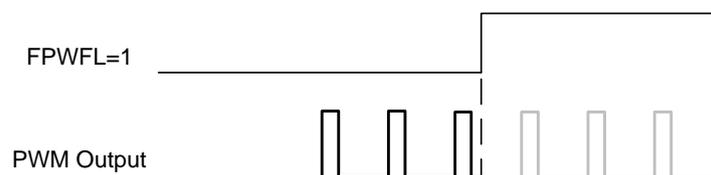
Fail detect function supports interrupt only if INT0 interrupt function is also enabled. When EX0=1 and PWFLEN=1, the program counter is pointed to 0x03 to execute ISR after INT0/PWMFL pin trigger event occurrence. Check FPWFL flag to identify if PWM event or not.
