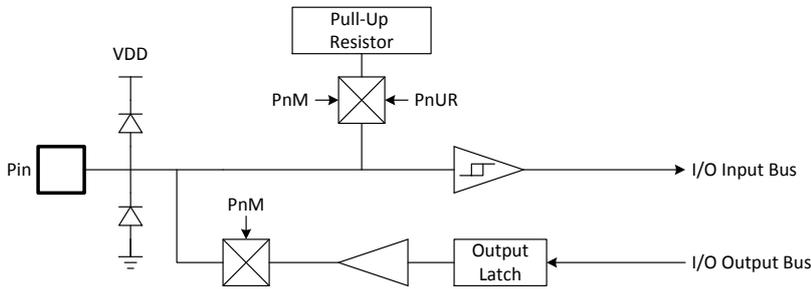
Bi-direction I/O Pin Shared with Specific Digital Input Function, e.g. INT2.
