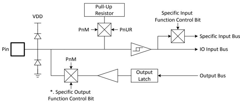
\*. Some specific functions switch I/O direction directly, not through PnM register.
