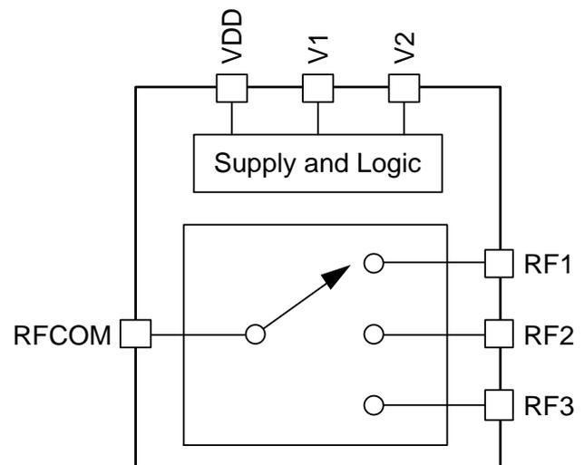
Figure 1. PS11103A Block Diagram
