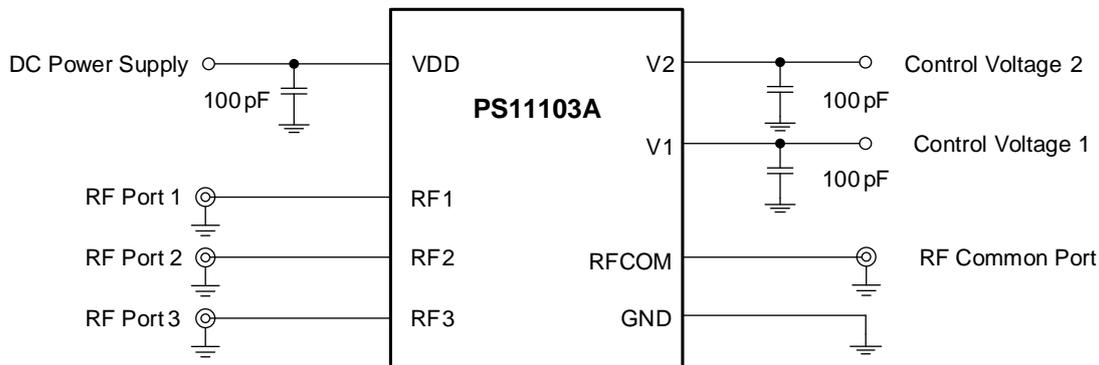
Figure 2. PS11103A Typical Application Circuit
