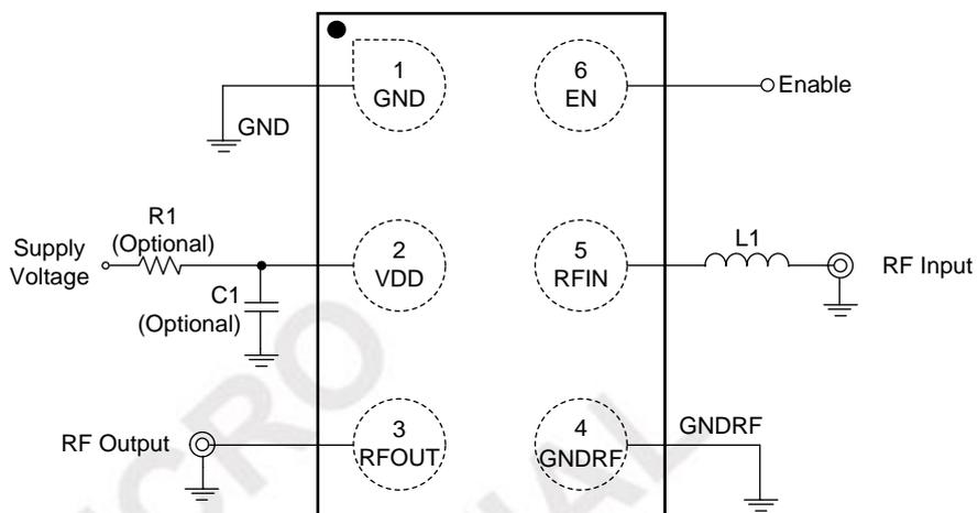
Figure 2. SGM13001A Typical Application Circuit
