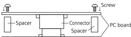
When connecting PC boards, take appropriate measures to prevent the connector from coming off.
