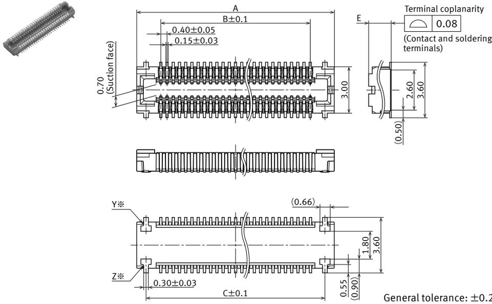
※Because the soldering terminal Y and Z are the unified structure, they are connected electrically.
