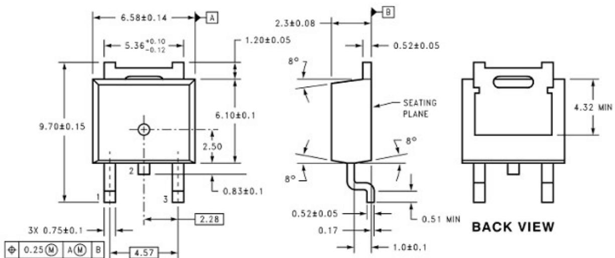
**DIMENSIONS ARE IN MILLIMETERS**
