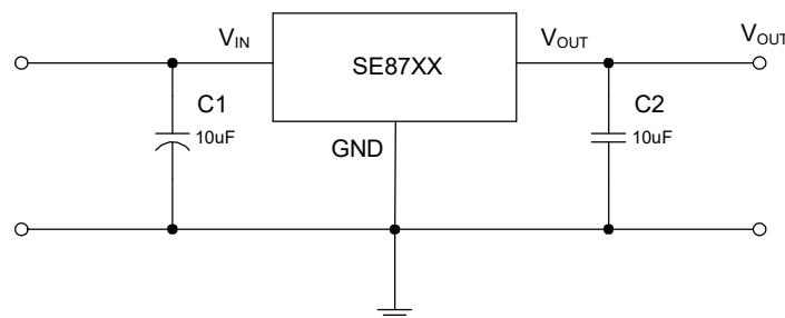
In plugging in application,  $C_{IN}$  is recommended to use  $10\mu F$  electrolytic capacitor or  $10\mu F$  MLCC with 2 ohm serial resistors to prevent large input voltage spike when plugging in. See APPLICATION INFORMATION for more information.
