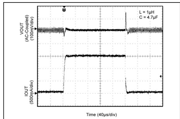
**FIGURE 2-28:** Load Transient (50 mA to 1.5A).
