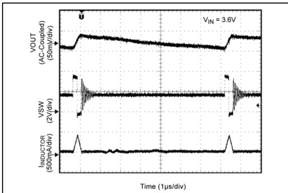
**FIGURE 2-19:** Switching Waveform Discontinuous Mode (Load = 10 mA).
