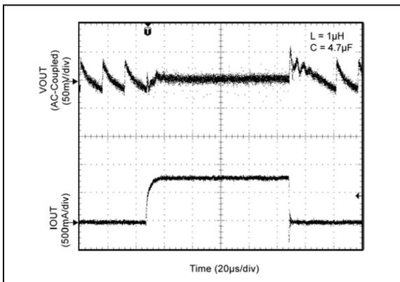
**FIGURE 2-26:** Load Transient (10 mA to 750 mA).
