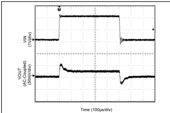
**FIGURE 2-32:** Line Transient (3.6V to 5.5V @ 1.5A Load).
