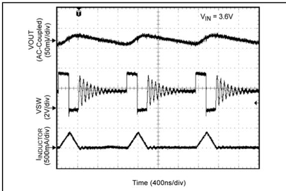
**FIGURE 2-20:** Switching Waveform Discontinuous Mode (Load = 50 mA).
