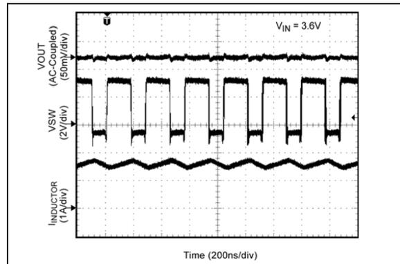
**FIGURE 2-23:** Switching Waveform Continuous Mode (Load = 1.5A)
