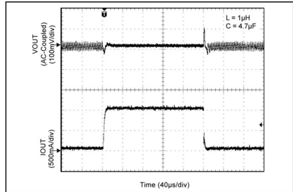
**FIGURE 2-27:** Load Transient (50 mA to 1A).
