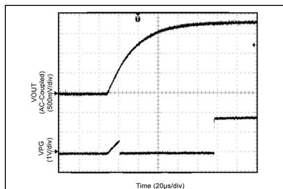
**FIGURE 2-34:** Start-Up and Power Good Waveform.
