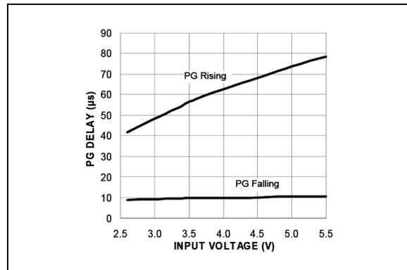
**FIGURE 2-11:** Power Good Delay Time vs. Input Voltage.
