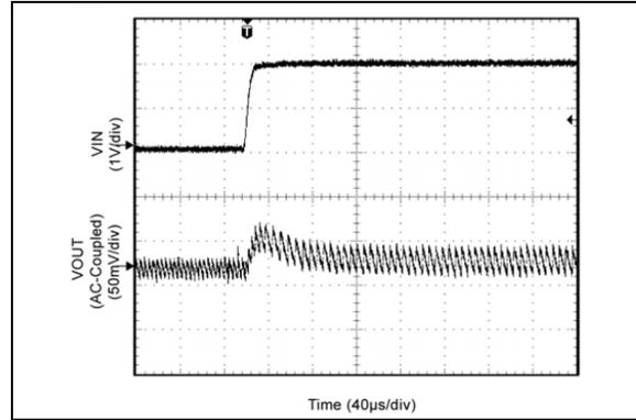
**FIGURE 2-33:** Line Transient (3.6V to 5.5V @ 20 mA Load).
