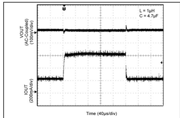
**FIGURE 2-29:** Load Transient (200 mA to 600 mA).
