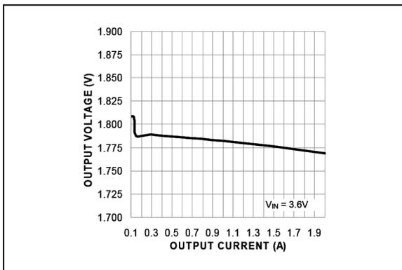
**FIGURE 2-9:** Output Voltage vs. Output Current (CCM).
