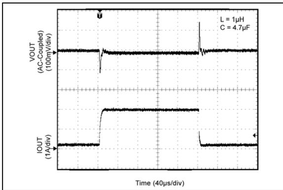
**FIGURE 2-31:** Load Transient (200 mA to 2A).
