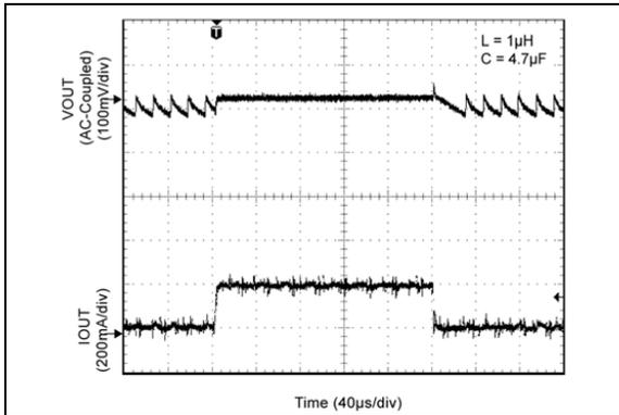
**FIGURE 2-24:** Load Transient (10 mA to 200 mA).
