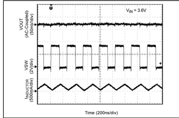
**FIGURE 2-21:** Switching Waveform Continuous Mode (Load = 150 mA).
