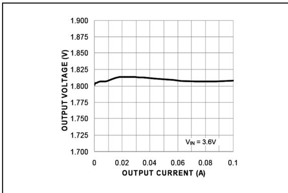
**FIGURE 2-8:** Output Voltage vs. Output Current (HLL).
