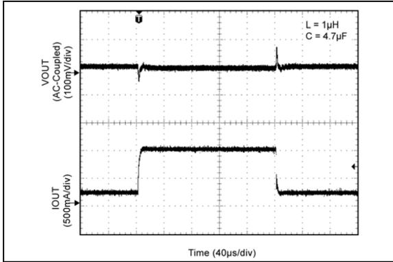
**FIGURE 2-30:** Load Transient (200 mA to 1A).
