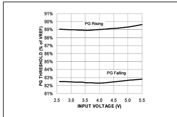
**FIGURE 2-12:** Power Good Thresholds vs. Input Voltage.
