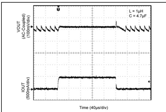
**FIGURE 2-25:** Load Transient (10 mA to 500 mA).
