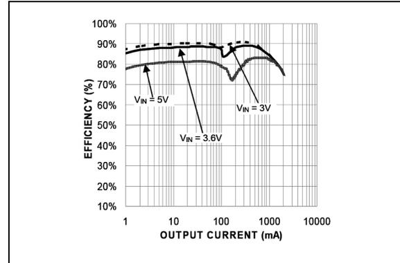
**FIGURE 5-2:** Efficiency Under Load
