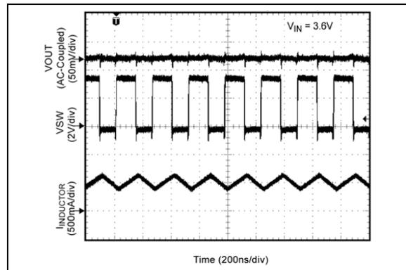
**FIGURE 2-22:** Switching Waveform Continuous Mode (Load = 500 mA).
