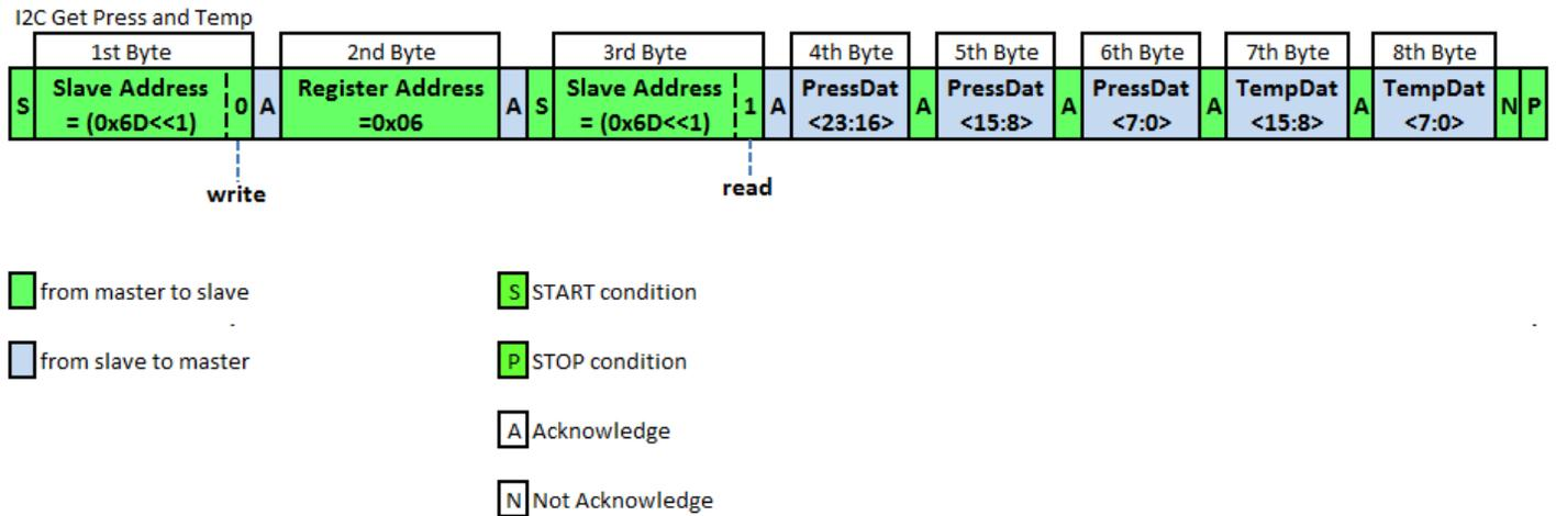
**FIGURE 2: 7-BIT SLAVE ADDRESS FOLLOWED BY THREE PRESSURE BYTES**
