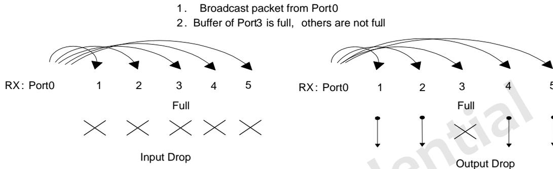
**Figure 20. Broadcast Input Drop vs. Output Drop**
