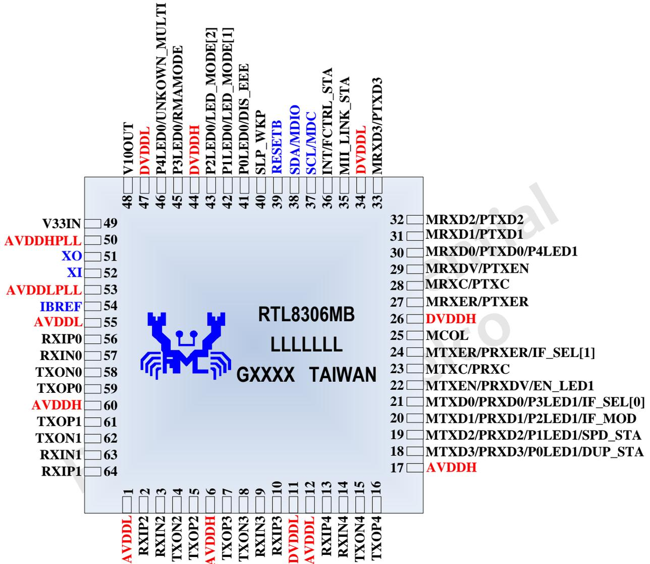
Figure 2. Pin Assignments
