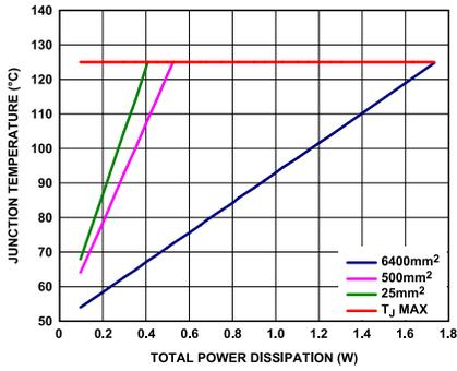
Figure 53. LFCSP,  $T_A = 50^\circ\text{C}$
