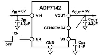
Figure 1. ADP7142 with Fixed Output Voltage, 5 V
