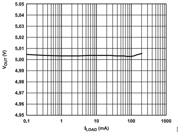
Figure 7. Output Voltage ( $V_{OUT}$ ) vs. Load Current ( $I_{LOAD}$ )
