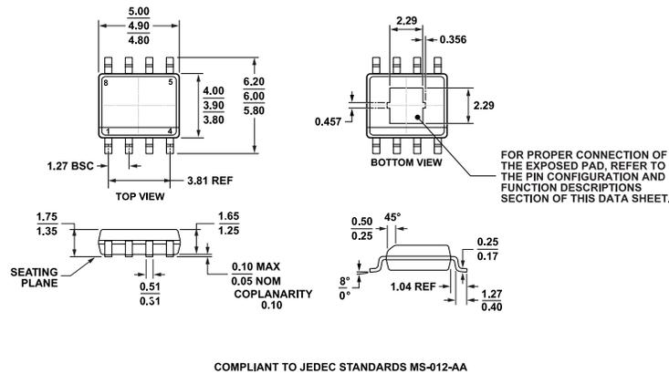
Figure 68. 8-Lead Standard Small Outline Package, with Exposed Pad [SOIC\_N\_EP]
