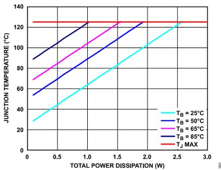
**Figure 62. SOIC Junction Temperature Rise, Different Board Temperatures**
