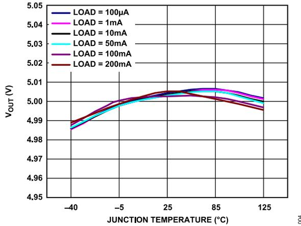
Figure 6. Output Voltage ( $V_{OUT}$ ) vs. Junction Temperature ( $T_J$ )
