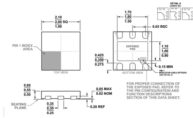
Figure 67. 6-Lead Lead Frame Chip Scale Package [LFCSP]
