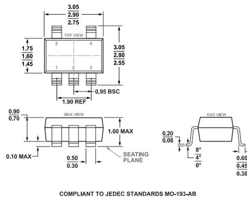
Figure 69. 5-Lead Thin Small Outline Transistor Package [TSOT]
