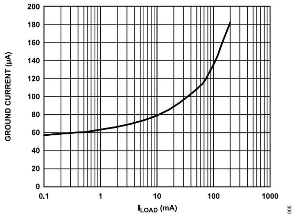
Figure 10. Ground Current ( $I_{GND}$ ) vs. Load Current ( $I_{LOAD}$ )
