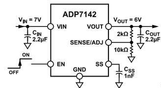
Figure 2. ADP7142 with 5 V Output Adjusted to 6 V
