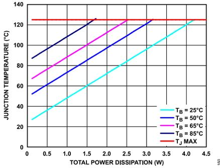
**Figure 61. LFCSP Junction Temperature Rise, Different Board Temperatures**
