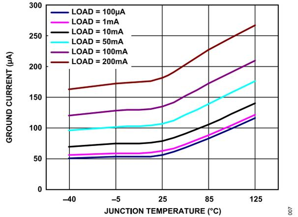
Figure 9. Ground Current ( $I_{GND}$ ) vs. Junction Temperature ( $T_J$ )
