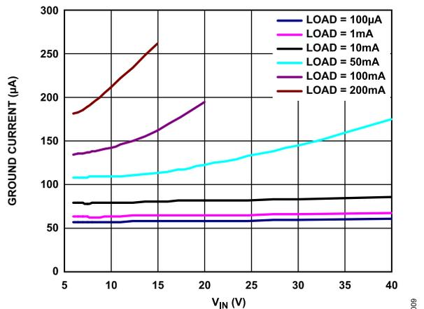
Figure 11. Ground Current ( $I_{GND}$ ) vs. Input Voltage ( $V_{IN}$ )
