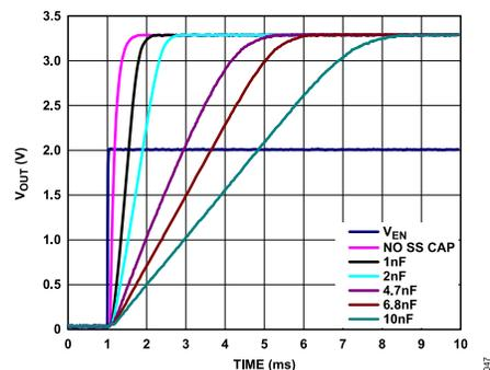
Figure 49. Typical Soft Start Behavior, Different  $C_{SS}$
