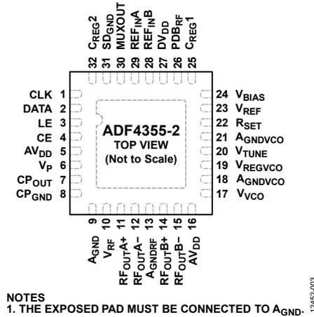
Figure 3. Pin Configuration
