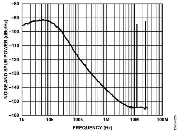
Figure 19. Fractional-N Spur Performance, W-CDMA Band,  $RF_{OUTA+} = 2113.5$  MHz,  $REF_{IN} = 122.88$  MHz, PFD = 61.44 MHz, Output Divide by 2 Selected, Loop Filter Bandwidth = 2 kHz, Channel Spacing = 20 kHz
