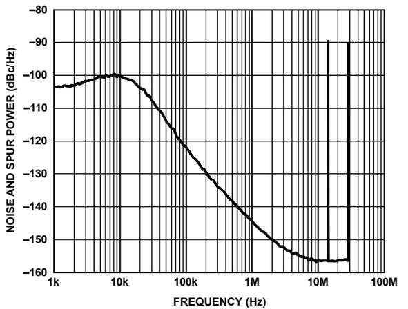
Figure 18. Fractional-N Spur Performance, GSM1800 Band,  $RF_{OUTA+} = 1550.2$  MHz,  $REF_{IN} = 122.88$  MHz, PFD = 61.44 MHz, Output Divide by 4 Selected, Loop Filter Bandwidth = 2 kHz, Channel Spacing = 20 kHz
