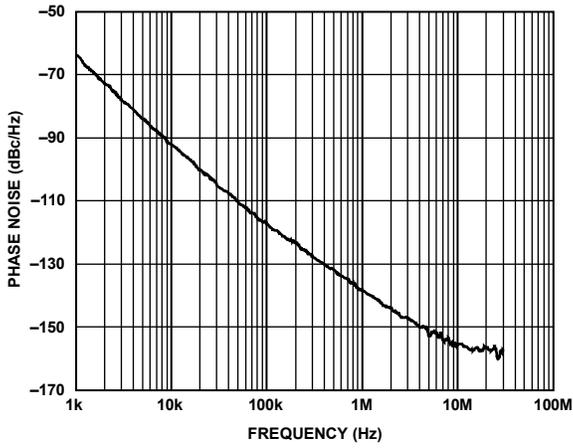
Figure 4. Open-Loop VCO Phase Noise, 3.4 GHz
