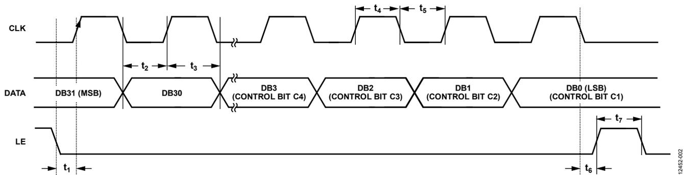
Figure 2. Timing Diagram
