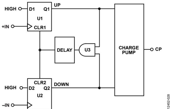
Figure 24. PFD Simplified Schematic
