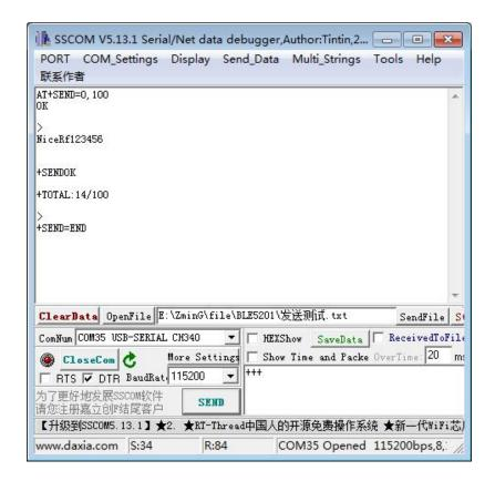
When a single packet sends a specific character string "+++\r\n", the one-way transparent transmission is ended early
