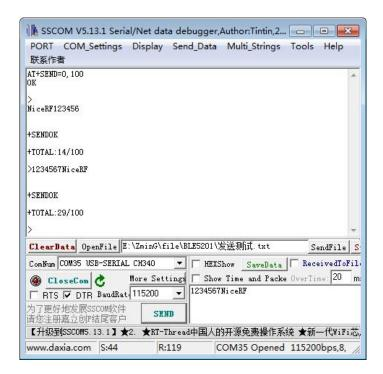
When the accumulated number of bytes sent reaches the preset maximum value, the one-way transparent transmission ends.
