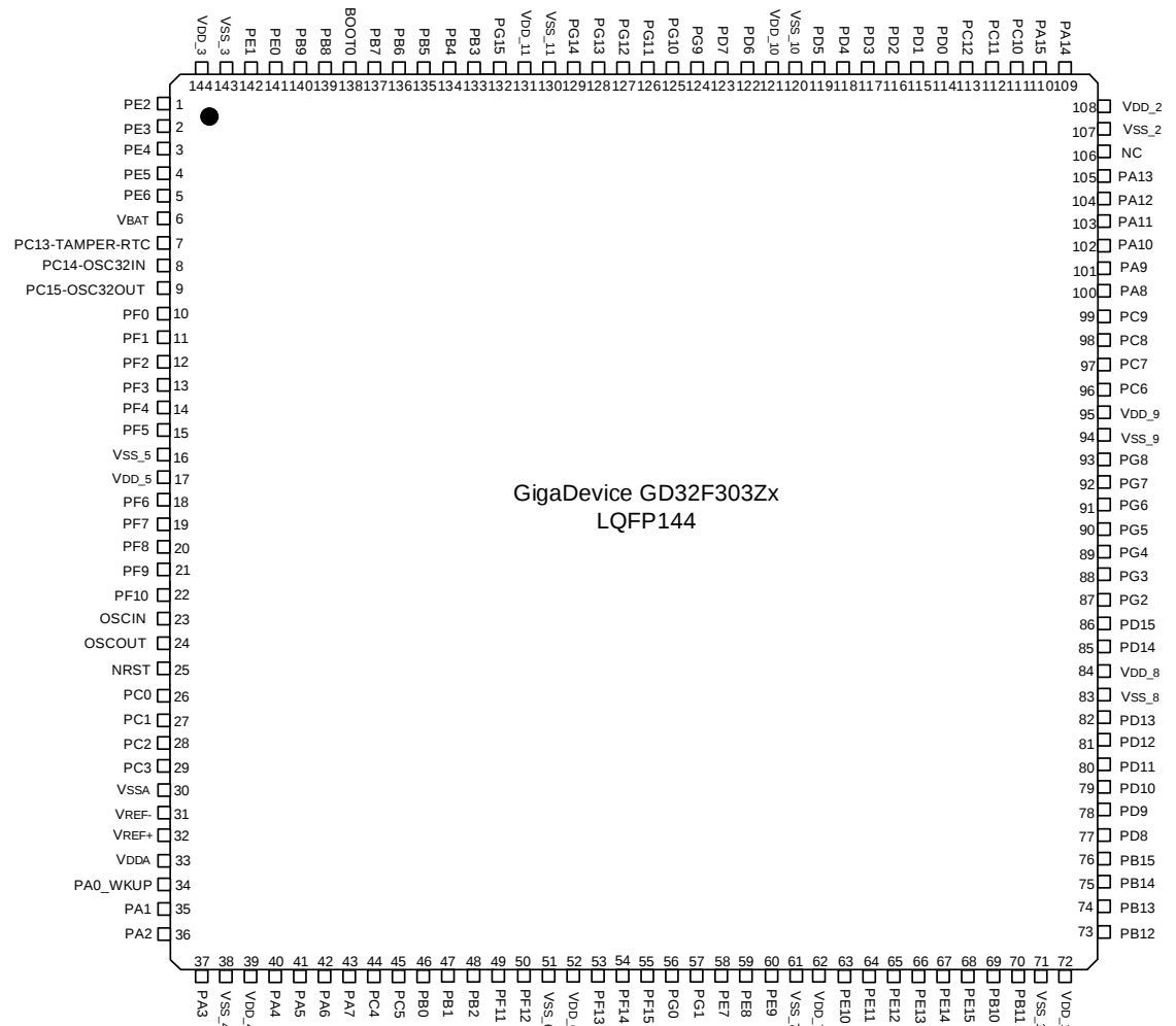
Figure 2-2. GD32F303Zx LQFP144 pinouts
