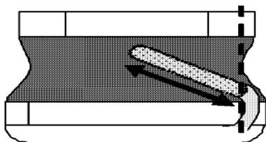
**Electrode appearance criterion for exposed wire**
