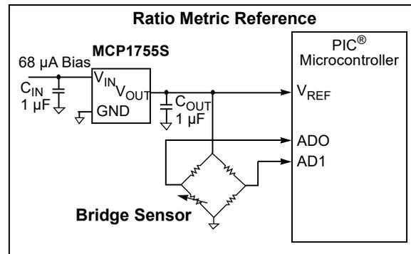
FIGURE 5-2: Using the MCP1755/MCP1755S as a Voltage Reference.
