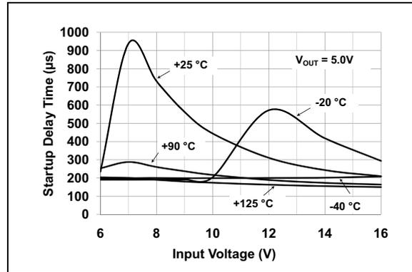
**FIGURE 2-34:** Start-up Delay from  $\overline{SHDN}$  to 90%  $V_{OUT}$ .
