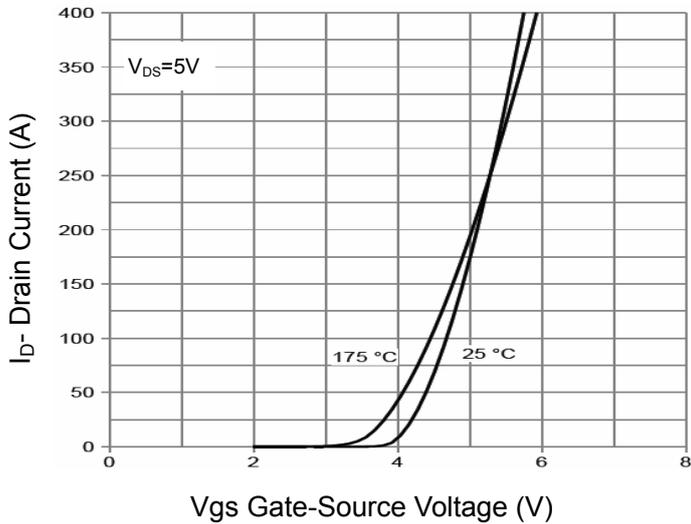
Figure 2 Transfer Characteristics
