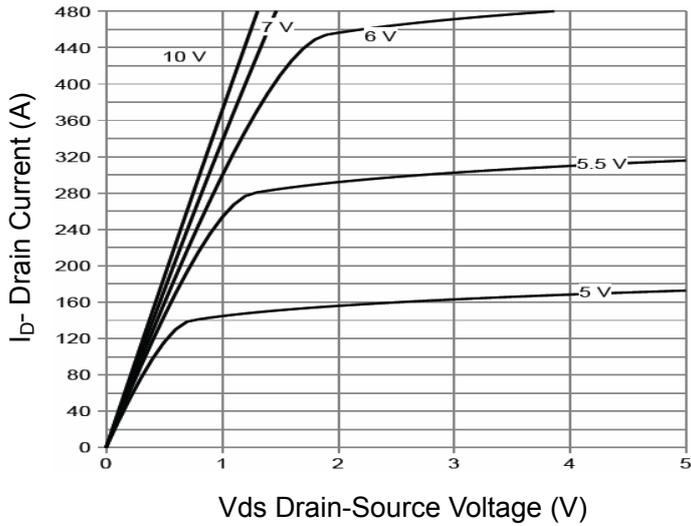
Figure 1 Output Characteristics
