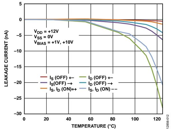
Figure 13. Leakage Current vs. Temperature, 12 V Single Supply
