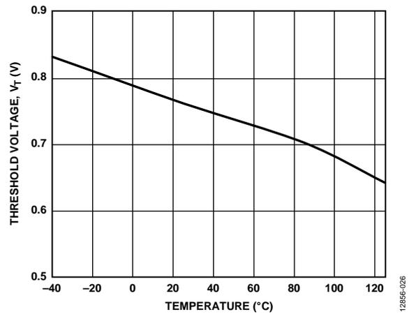
Figure 27. Threshold Voltage ( $V_T$ ) vs. Temperature
