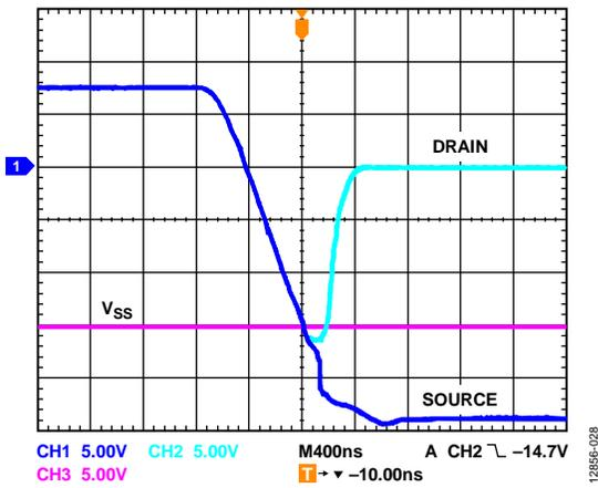
Figure 29. Drain Output Response to Negative Overvoltage
