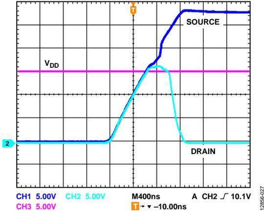
Figure 28. Drain Output Response to Positive Overvoltage
