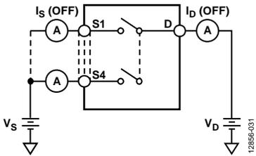
Figure 32. Off Leakage
