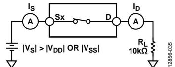
Figure 36. Switch Overvoltage Leakage
