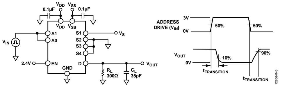
Figure 47. Address to Output Switching Times,  $t_{TRANSITION}$
