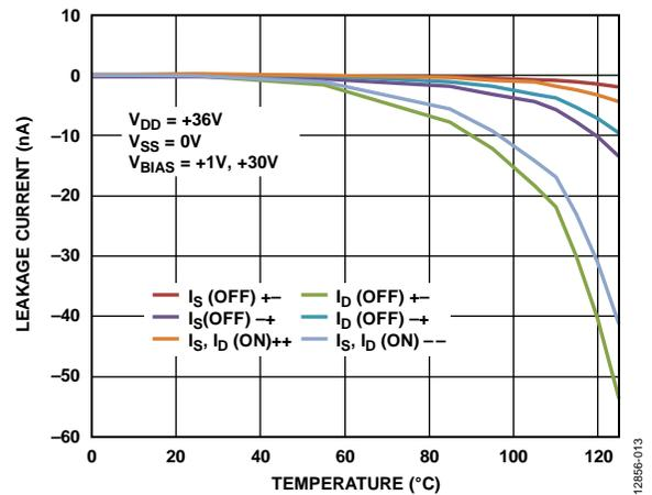
Figure 14. Leakage Current vs. Temperature, 36 V Single Supply
