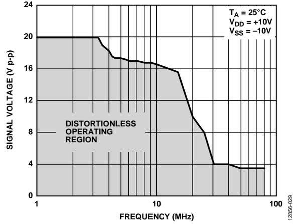
Figure 30. Large Signal Voltage Tracking vs. Frequency
