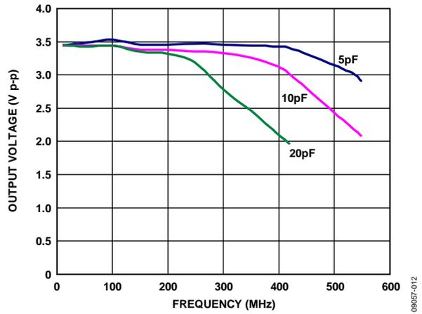
Figure 14. Peak-to-Peak Output Voltage vs. Frequency, CMOS
