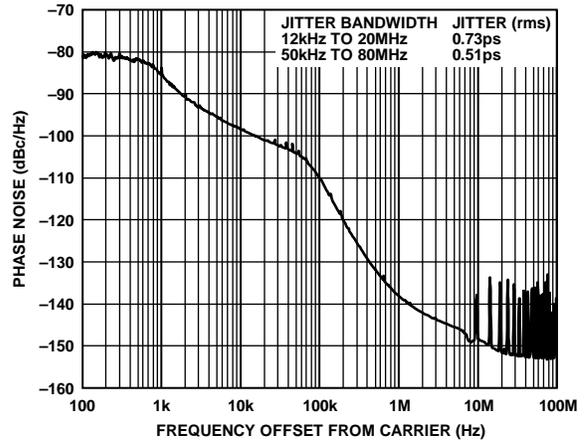
Figure 6. Phase Noise ( $f_{REF} = 77.76$  MHz,  $f_{OUT1} = 622.08$  MHz)
