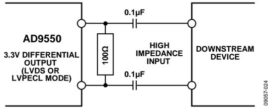
Figure 21. AC-Coupled LVDS or LVPECL Output Driver
