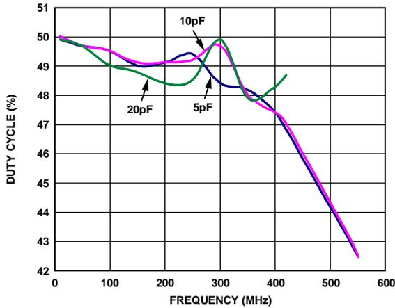
Figure 16. Duty Cycle vs. Output Frequency, CMOS
