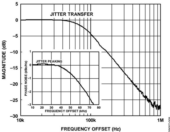
Figure 11. Jitter Transfer, Loop Bandwidth = 75 kHz
