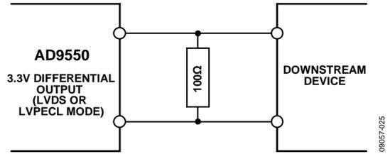
Figure 22. DC-Coupled LVDS or LVPECL Output Driver
