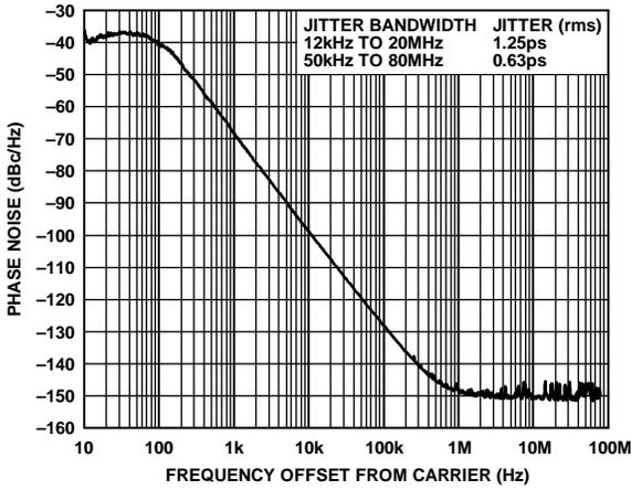
Figure 5. Phase Noise ( $f_{REF} = 61.44$  MHz,  $f_{OUT1} = 122.88$  MHz)
