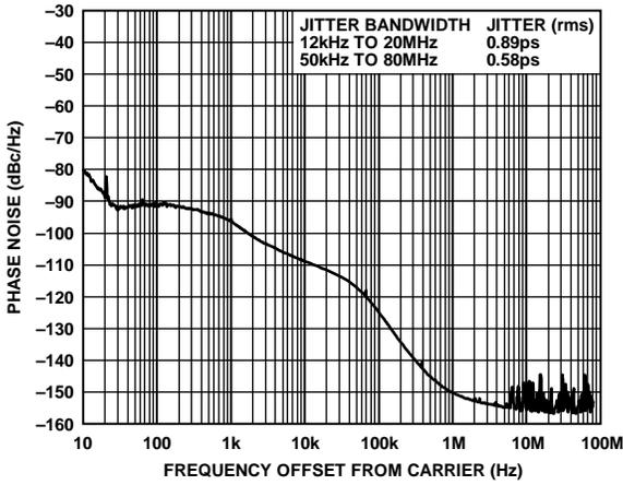
Figure 3. Phase Noise ( $f_{REF} = 25$  MHz,  $f_{OUT1} = 125$  MHz)
