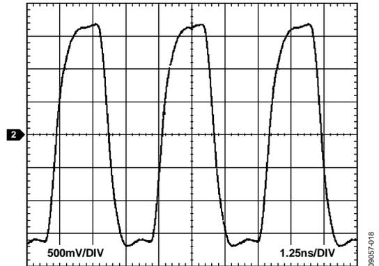
Figure 20. Typical Output Waveform, CMOS (250 MHz, 10 pF Load)
