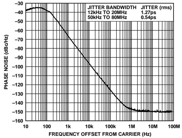
Figure 8. Phase Noise ( $f_{REF} = 8$  kHz,  $f_{OUT1} = 155.52$  MHz)
