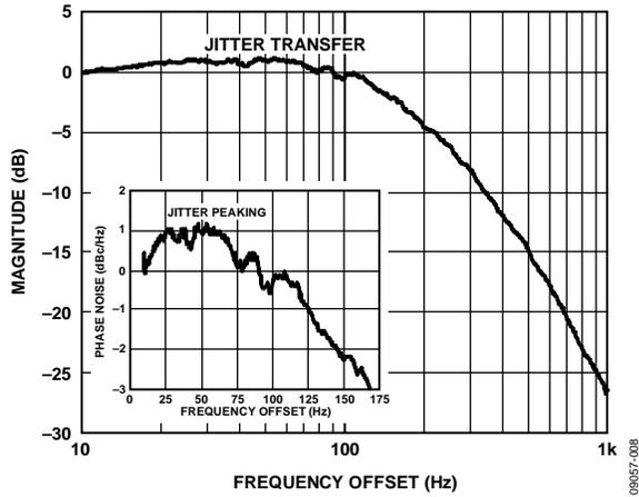
Figure 9. Jitter Transfer, Loop Bandwidth = 170 Hz
