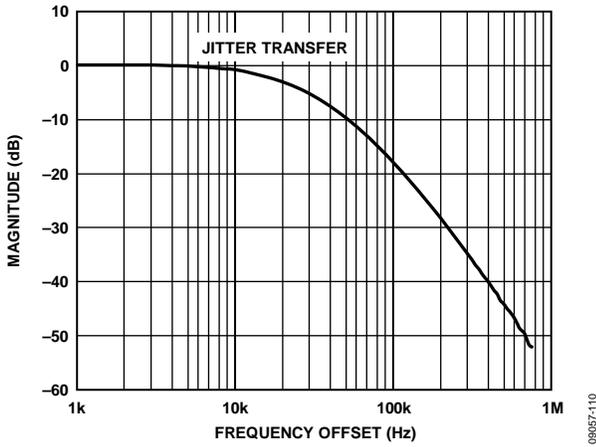
Figure 10. Jitter Transfer, Loop Bandwidth = 20 kHz
