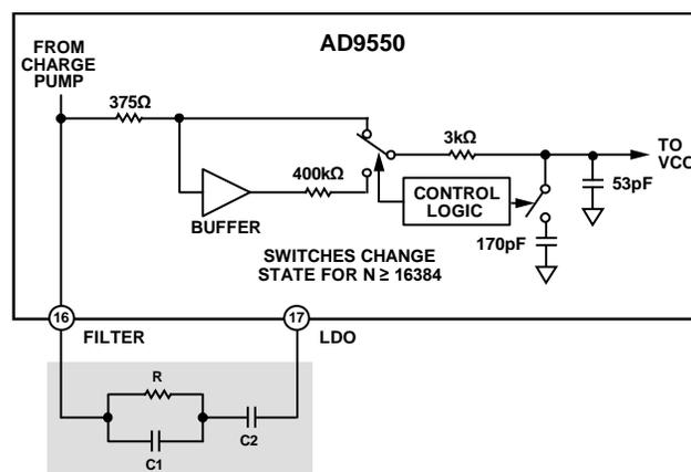
Figure 24. External Loop Filter
