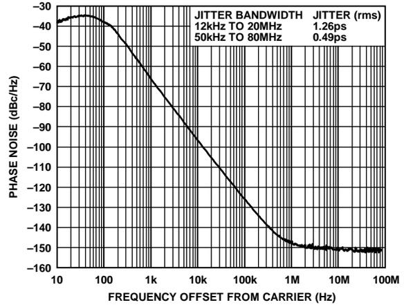
Figure 7. Phase Noise ( $f_{REF} = 19.44$  MHz,  $f_{OUT1} = 155.52$  MHz)
