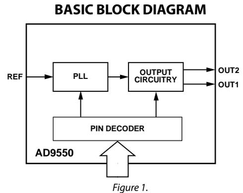
15 possible input frequencies to a list of 52 possible output frequency pairs (OUT1 and OUT2).
