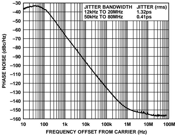
Figure 4. Phase Noise ( $f_{REF} = 25$  MHz,  $f_{OUT1} = 156.25$  MHz)
