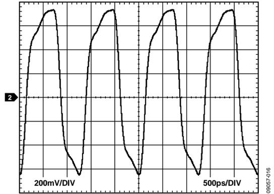
Figure 18. Typical Output Waveform, LVPECL (800 MHz)
