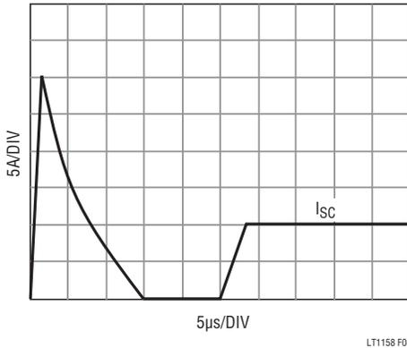
Figure 8. Top MOSFET Short-Circuit Turn-On current
