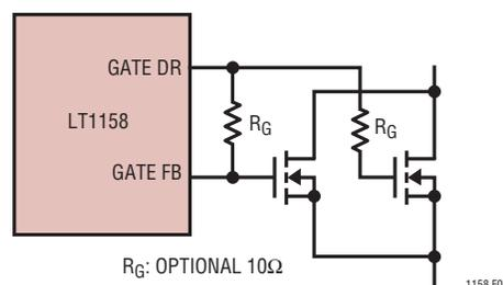
Figure 1. Paralleling MOSFETs
