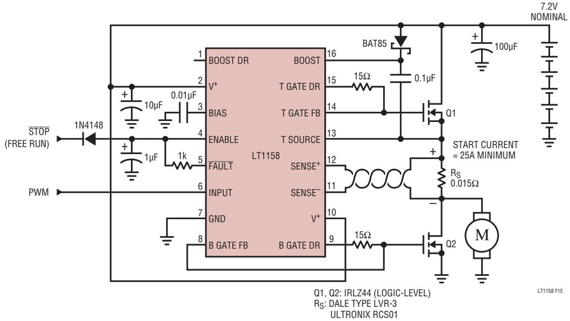
Figure 15. High Efficiency 6-Cell NiCd Protected Motor Drive
