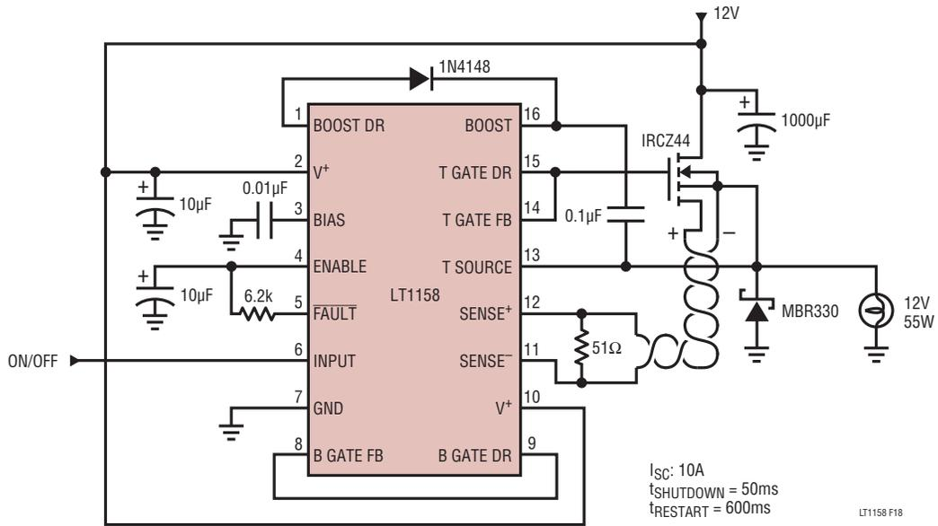
**Figure 18. High Current Lamp Driver with Short-Circuit Protection**
