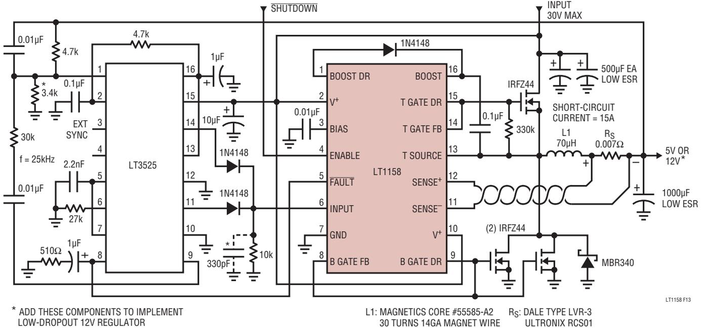
Figure 13. 90% Efficiency 24V to 5V 10A Switching Regulator
