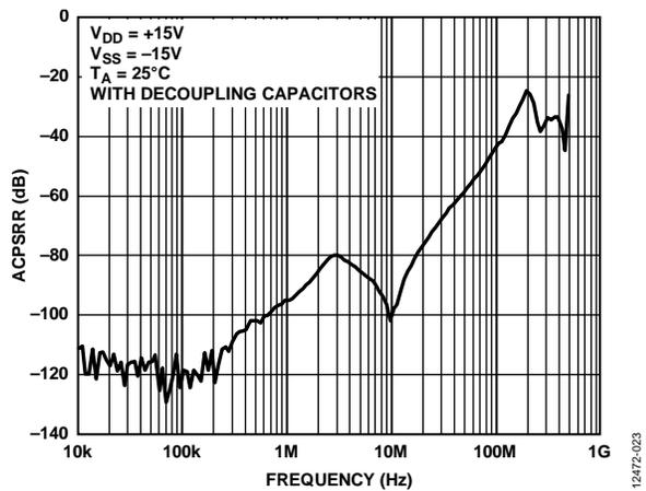
Figure 24. ACPSRR vs. Frequency,  $\pm 15$  V Dual Supply
