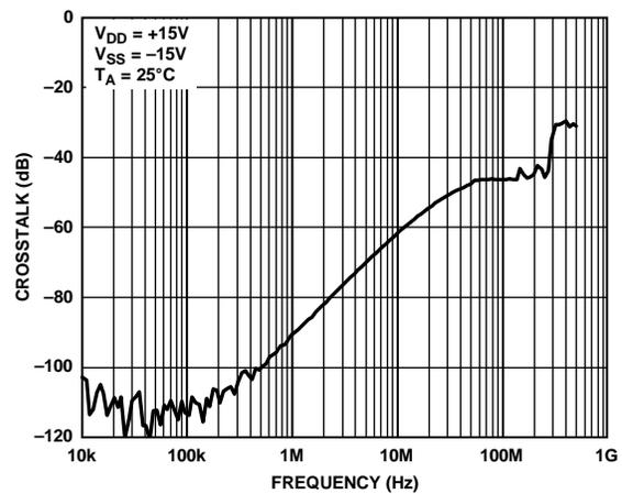
Figure 21. Crosstalk vs. Frequency, ±15 V Dual Supply
