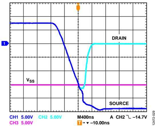
Figure 30. Drain Output Response to Negative Overvoltage
