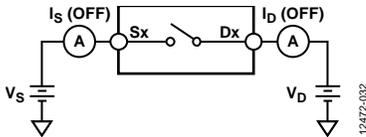
Figure 33. Off Leakage
