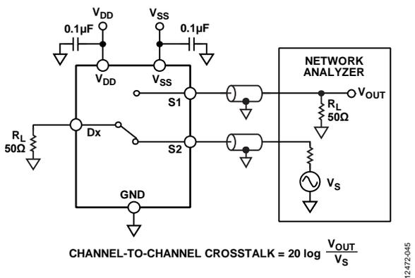
Figure 36. Channel-to-Channel Crosstalk
