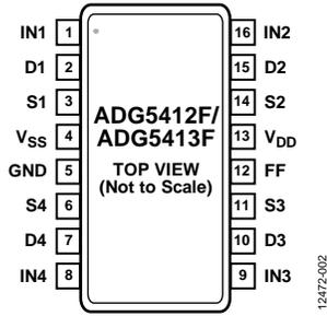
Figure 3. TSSOP Pin Configuration
