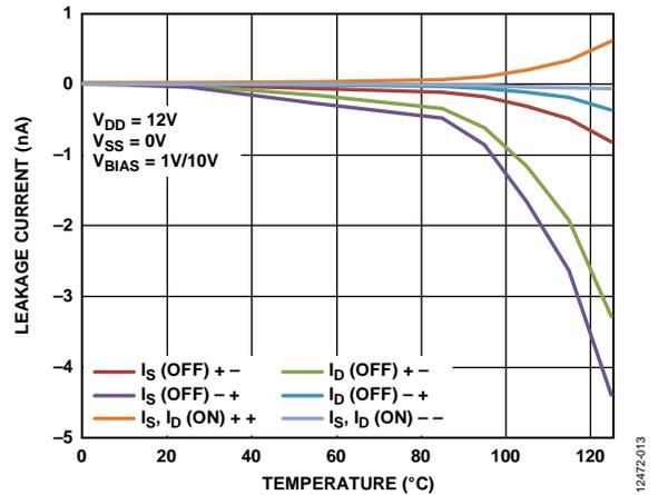
Figure 14. Leakage Current vs. Temperature, 12 V Single Supply
