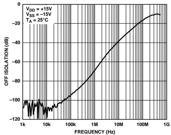
Figure 20. Off Isolation vs. Frequency, ±15 V Dual Supply
