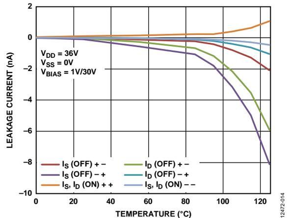
Figure 15. Leakage Current vs. Temperature, 36 V Single Supply
