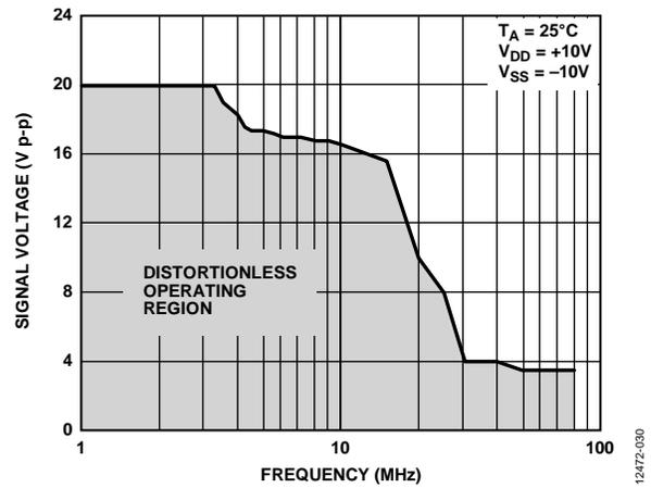
Figure 31. Large Voltage Signal Tracking vs. Frequency
