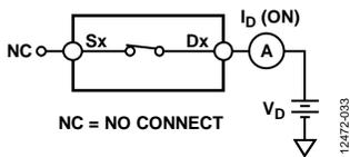
Figure 34. On Leakage
