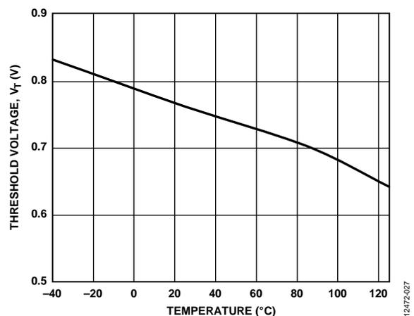
Figure 28. Threshold Voltage ( $V_T$ ) vs. Temperature
