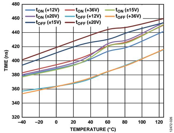
Figure 27.  $t_{ON}$ ,  $t_{OFF}$  Times vs. Temperature
