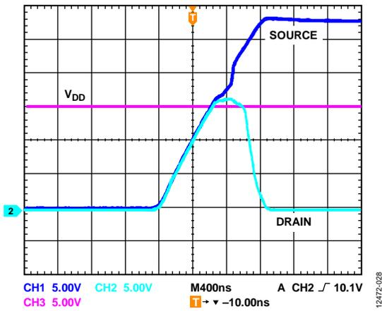
Figure 29. Drain Output Response to Positive Overvoltage
