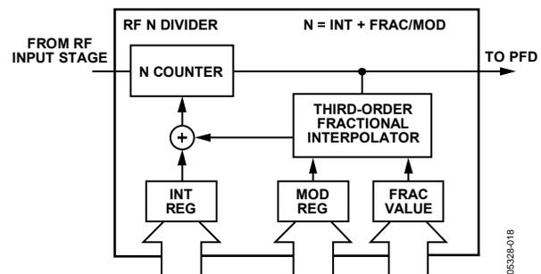
Figure 22. Fractional-N Divider
