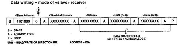
2. **Mode of «slave» receiver (write mode from JHT1307):** The first byte is received and processed as in the mode of the «slave» receiver. However, in this mode the direction bit will signify, that the transmission direction is changed. JHT1307 sends the serial data by SDA, the cycle pulses - by SCL. statuses START and STOP are understood as the beginning and end of the consecutive transmission. The address byte is the first byte, received after occurrence of the status START,
