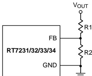
Figure 4. Output Voltage Setting
