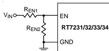
Figure 3. Resistor Divider for Lockout Threshold Setting
