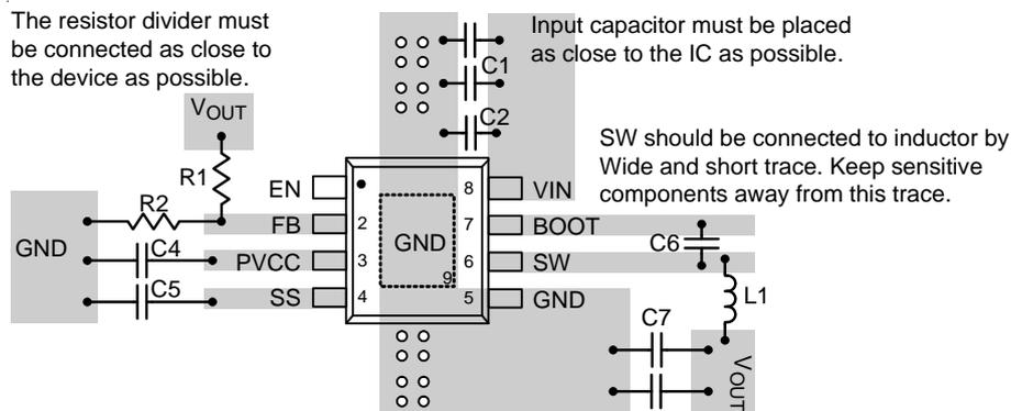
(c). For SOP-8 (Exposed) Package
