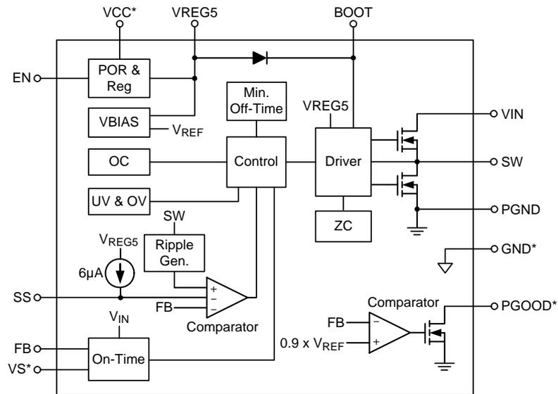
\* : VCC pin for TSSOP-14 (Exposed Pad) only. VS pin for TSSOP-14 (Exposed Pad) only.
