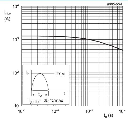
Fig. 4b. Non-repetitive peak forward current as a function of pulse width; sinusoidal waveform; maximum values; Standard diode
