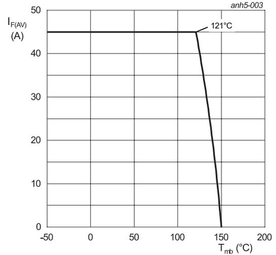
Fig. 3b. Forward current as a function of mounting base temperature; maximum values; Standard diode
