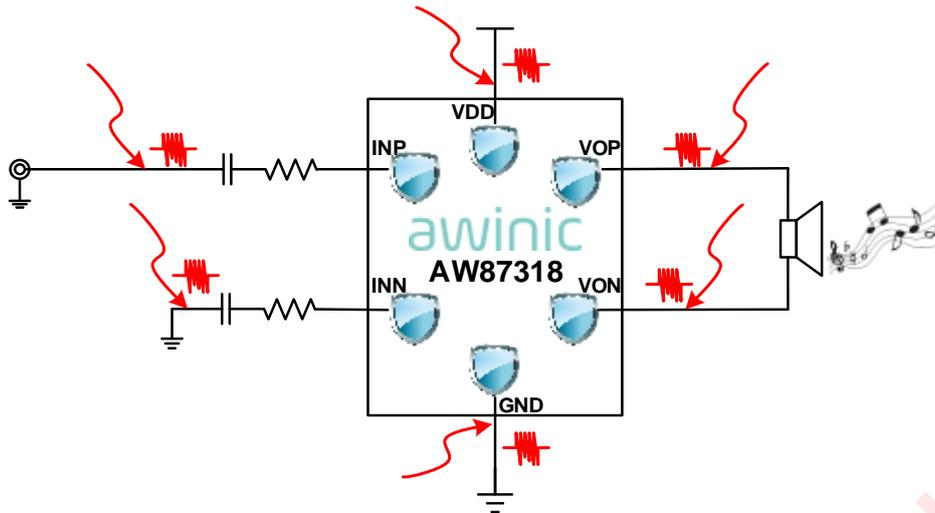
Figure 15 AW87318 Rejection of RF Noise
