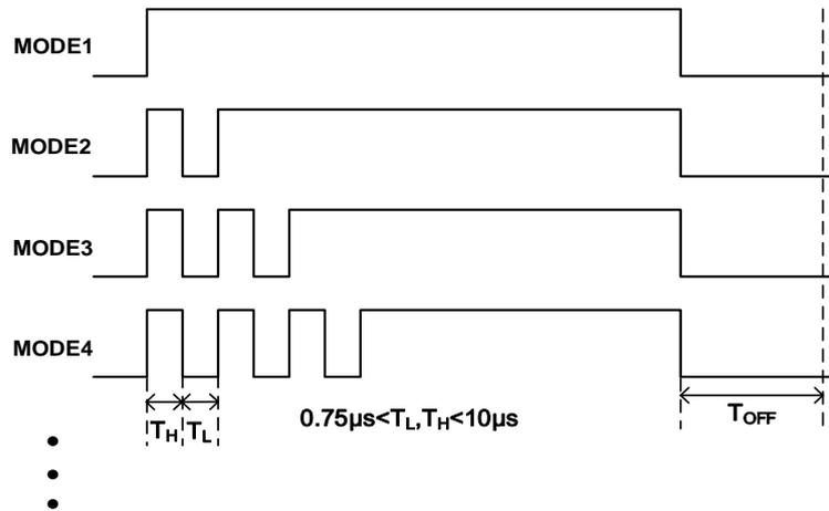
Figure 13 Working Mode Setting through One-Wire Pulse Control
