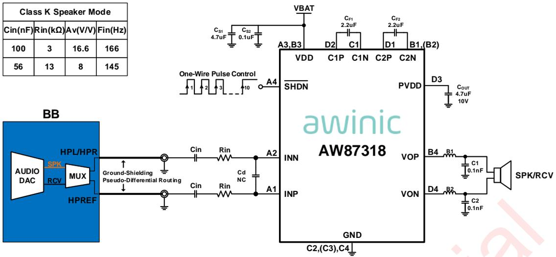
Figure 4 AW87318 Speaker Mode Application Diagram (Note 1)
