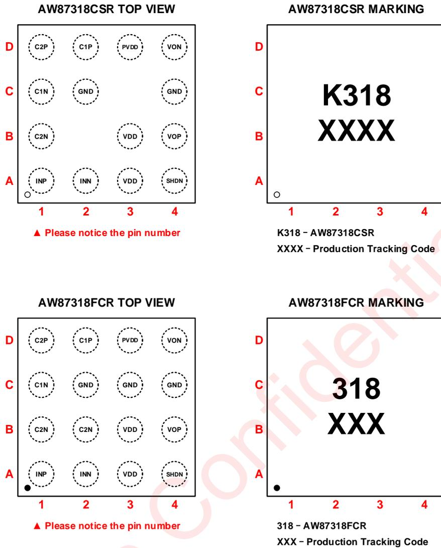
Figure 2 AW87318CSR and AW87318FCR Pin Diagram Top View and Device Marking
