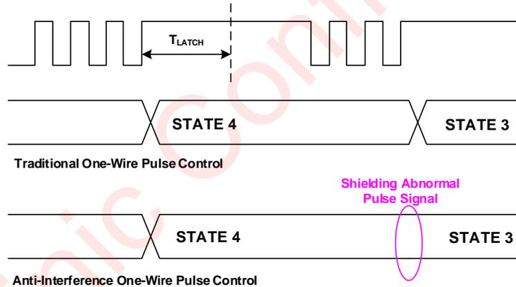
Figure 12 Anti-Interference One-Wire Pulse Control Functional Diagram
