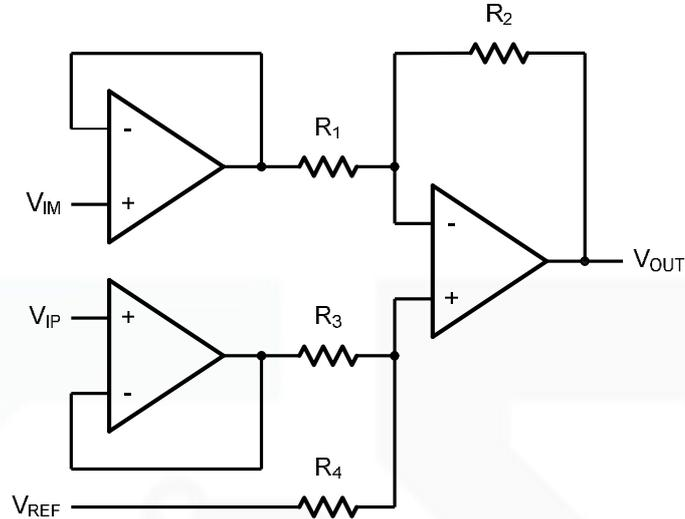
Figure 6. Instrument Amplifier
