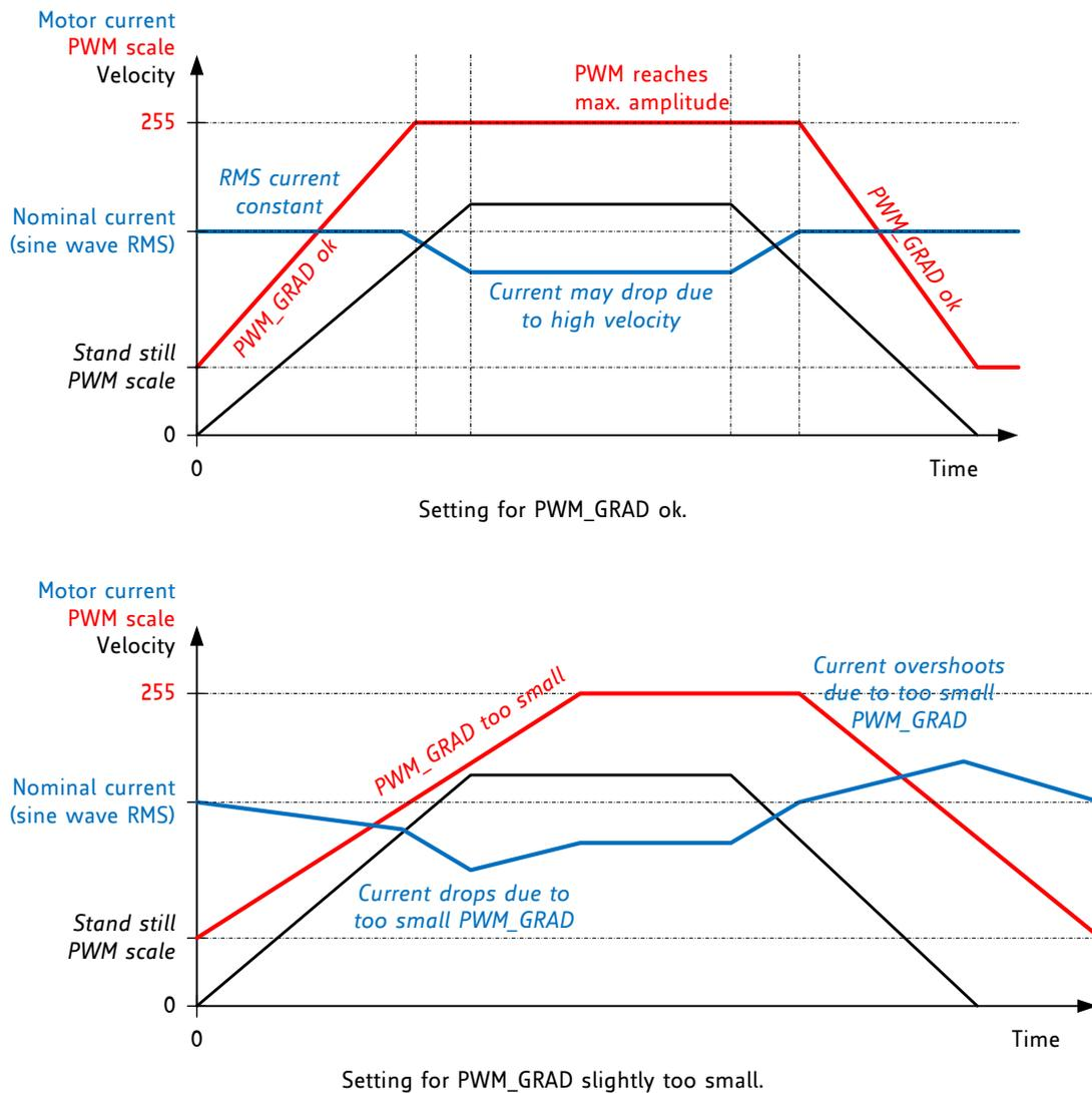
**Figure 7.4 Good and too small setting for PWM\_GRAD**
