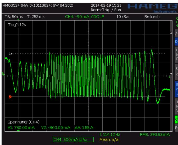
Figure 7.3 Scope shot: too small setting for  $PWM\_GRAD$
