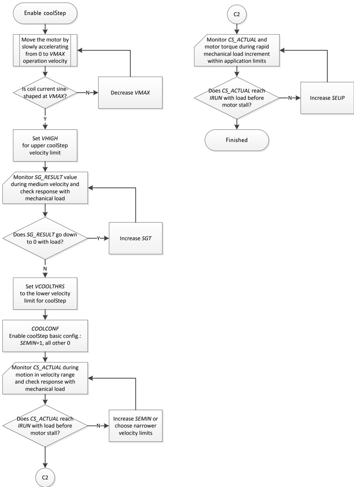
**Figure 14.4 Enabling coolStep (only in combination with spreadCycle)**
