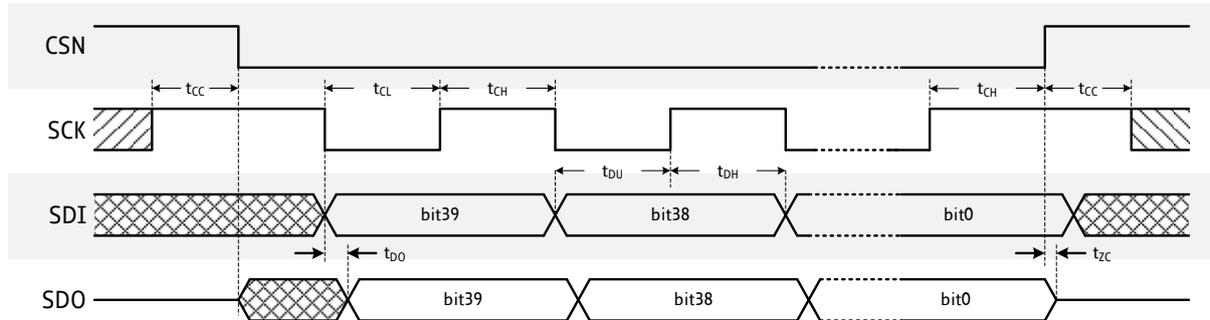
Figure 4.1 SPI timing
