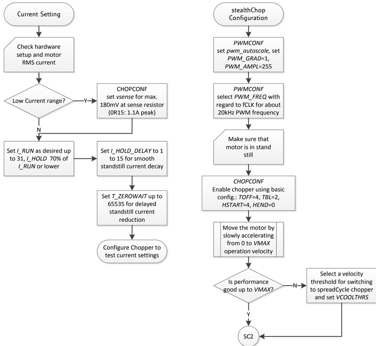
Figure 14.1 Current setting and first steps with stealthChop
