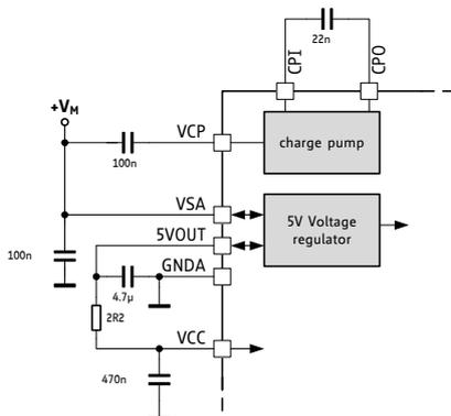
Figure 3.5 RC-Filter on VCC for reduced ripple
