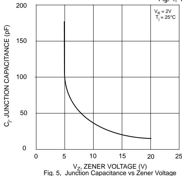
Fig. 5, Junction Capacitance vs Zener Voltage
