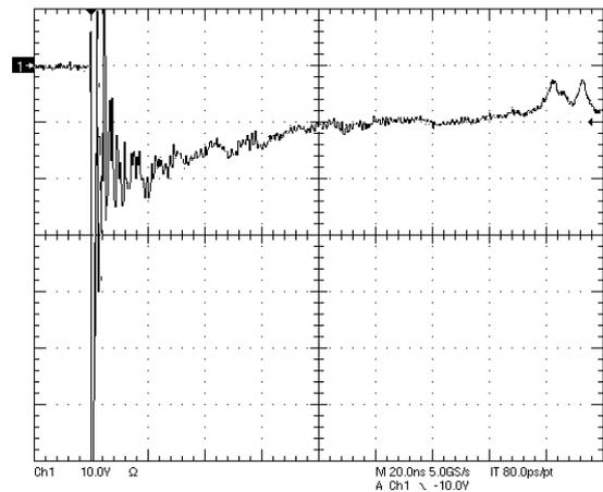
**Figure 2. ESD Clamping Voltage Screenshot
