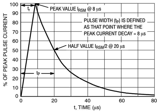
Figure 4. 8 X 20  $\mu s$  Pulse Waveform
