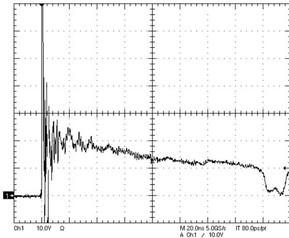
**Figure 1. ESD Clamping Voltage Screenshot
