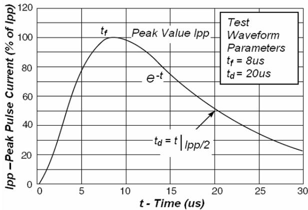
Fig1. Pulse Waveform
