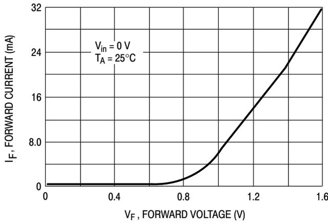
**Figure 12. Clamp Diode Forward Current versus Voltage**
