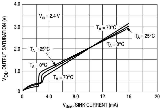
**Figure 10. MC3X164-3 Reset Output Saturation versus Sink Current**
