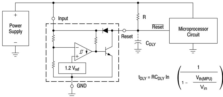
A time delayed reset can be accomplished with the addition of  $C_{DLY}$ . For systems with extremely fast power supply rise times ( $< 500$  ns) it is recommended that the  $RC_{DLY}$  time constant be greater than  $5.0 \mu\text{s}$ .  $V_{th(MPU)}$  is the microprocessor reset input threshold.
