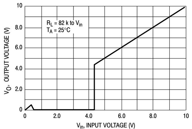
Figure 3. MC3X164-5  $\overline{\text{Reset}}$  Output Voltage versus Input Voltage
