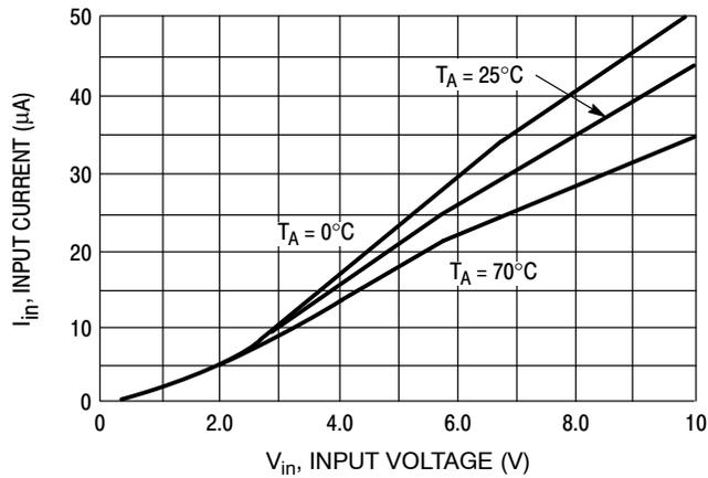
**Figure 8. MC3X164-3 Input Current versus Input Voltage**
