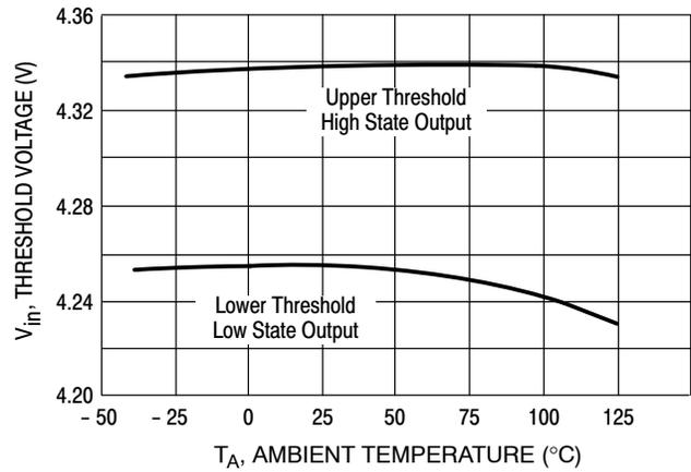
**Figure 7. MC3X164-5 Comparator Threshold Voltage versus Temperature**
