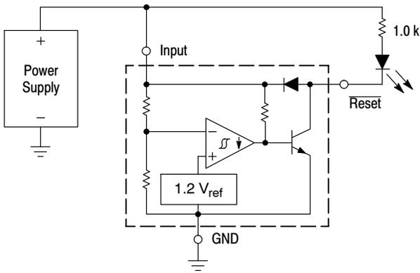
**Figure 16. Voltage Monitor**
