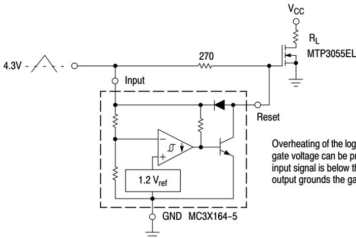
Overheating of the logic level power MOSFET due to insufficient gate voltage can be prevented with the above circuit. When the input signal is below the 4.3 V threshold of the MC3X164-5, its output grounds the gate of the L<sup>2</sup> MOSFET.
