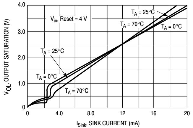
**Figure 11. MC3X164-5 Reset Output Saturation versus Sink Current**
