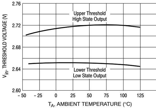
**Figure 6. MC3X164-3 Comparator Threshold Voltage versus Temperature**
