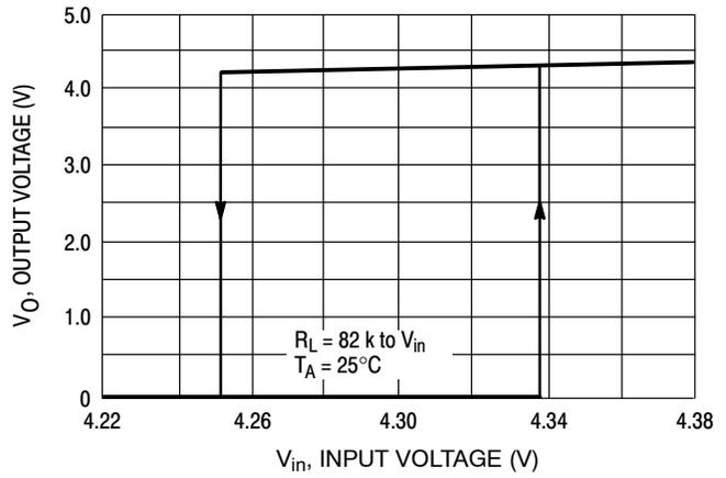
**Figure 5. MC3X164-5  $\overline{\text{Reset}}$  Output Voltage versus Input Voltage**
