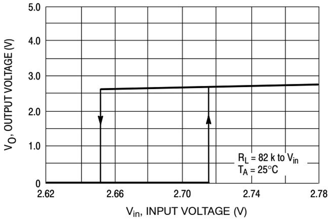
**Figure 4. MC3X164-3  $\overline{\text{Reset}}$  Output Voltage versus Input Voltage**
