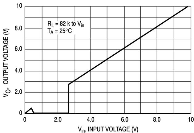
Figure 2. MC3X164-3  $\overline{\text{Reset}}$  Output Voltage versus Input Voltage
