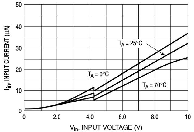
**Figure 9. MC3X164-5 Input Current versus Input Voltage**
