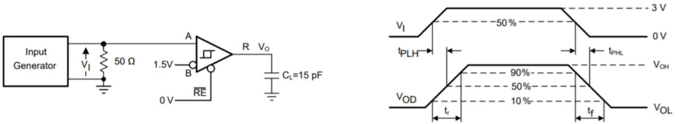
Figure 5. Receiver Propagation Delay and Data rate
