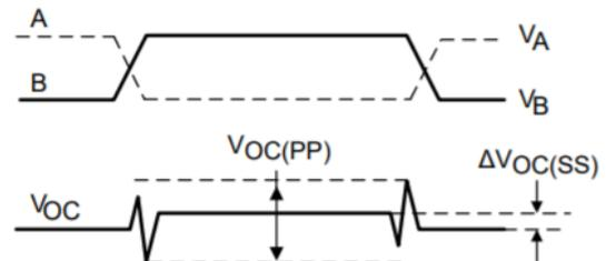
Figure 4. Driver Propagation Delay and Rise/Fall Time Measurement
