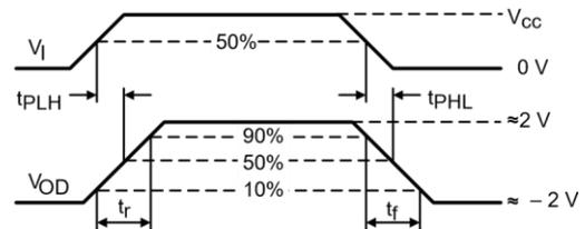
Figure 2. Driver Propagation Delay and Differential Transition Times
