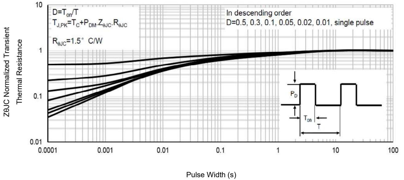
Fig13 . Normalized Maximum Transient Thermal Impedance
