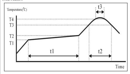
高温回流焊 Solder Heat-Resistance Test
