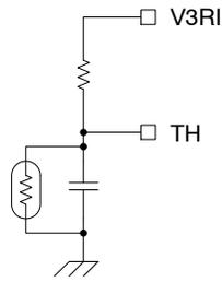
**Figure 14. Example Circuit for External Temperature Sensing**
