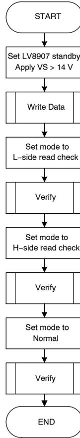
**Figure 22. OTP Memory Write and Verify Flow**
