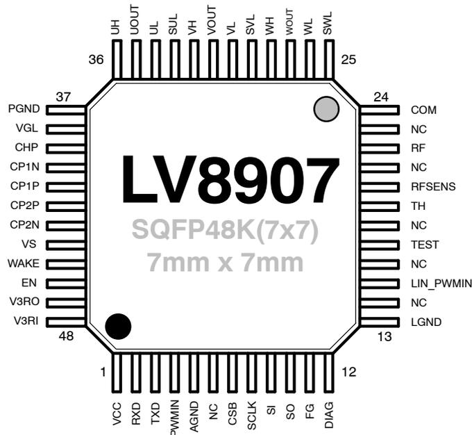
Figure 4. LV8907 Pinout
