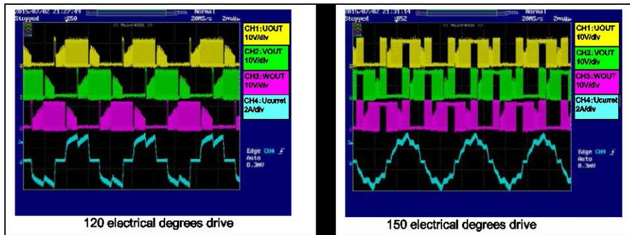
**Figure 7. Trapezoidal vs. Sinusoidal Drive @ 50% Duty Cycle**
