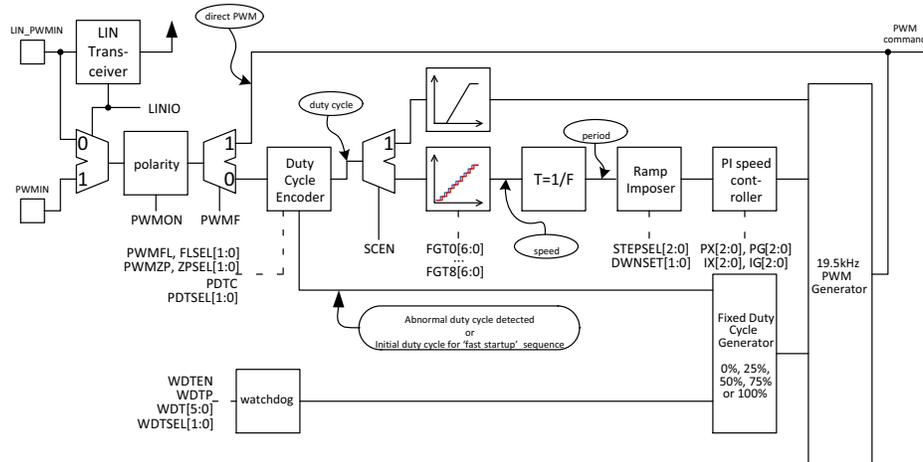
Figure 12. PWM Command Flow and Related Registers
