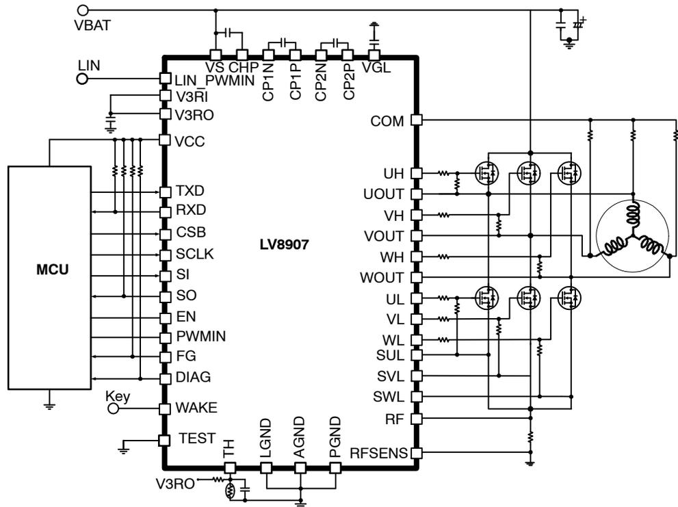
Figure 3. Example of LIN Based Control Configuration
