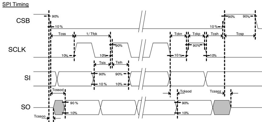
**Figure 16. SPI Timing Chart**
