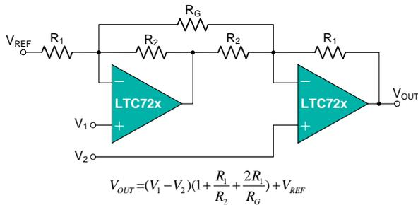
Figure 9. Instrumentation Amplifier
