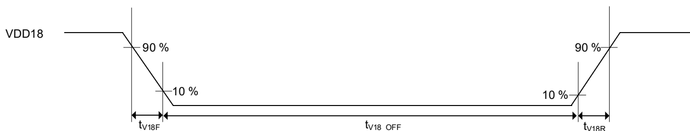
Figure 10. Power Supply Rise and Fall Time
