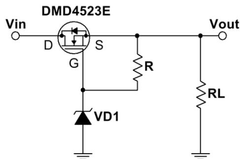
Figure 8. The DMD4523E for overcurrent and overvoltage protection
