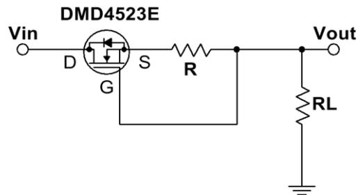
Figure 7. The DMD4523E is used for current limiting
