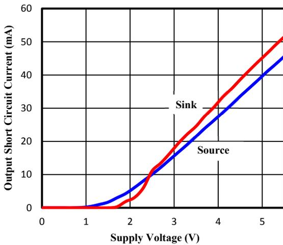
Figure 3. Output Short Circuit Current vs. Supply Voltage
