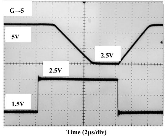
Figure 14. Negative Overload Recovery Time
