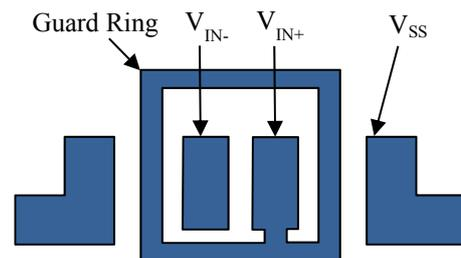
Figure 24. Example Guard Ring Layout for Inverting Gain
