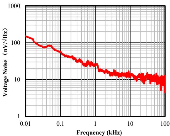
Figure 11. Input Voltage Noise Spectral Density vs. Frequency
