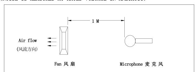
(在背景噪音不超过18dB (A) 的无响室内,将待测风扇通入额定的工作电压,悬掉入空中,将麦克风放于风扇同一平面且离待测风扇进风口一米处进行测试其 B&K 值)Noise is measured rated voltage in free air in anechoic chamber with B&K sound IeveI meter with microphone at a distance of one meter from the fan intake. The background noise is 18Db(A) max。
